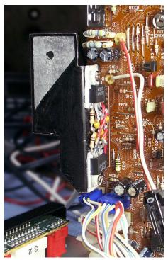
amps have local feedback which sets their gain, there should not be a need for readjustments, due to the replacement.
