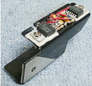
use the drawing <u>at right</u>. (Below, we will cover a slightly different version for use with the DIY replacement circuit.) The arrows show how the sides are bent up to form a U-shape. Aluminum, 0.0625" sheet metal is the material. The servo amp is mounted on the opposite side from the one we are viewing. The slot and hole work with the existing amp mounting hardware which you can see in the upper pic on page-2.
