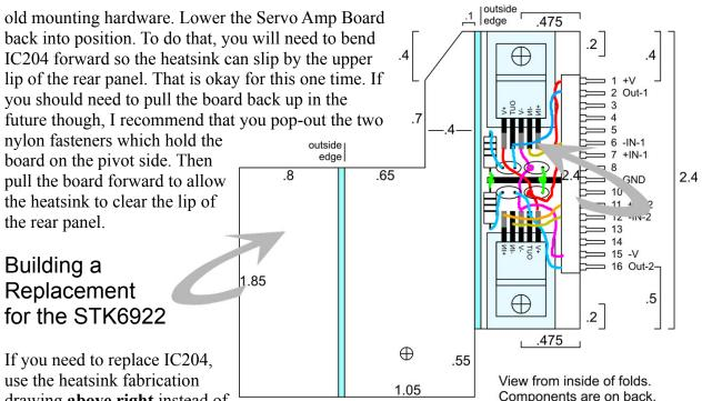
drawing above right instead of the one on page-5. This one substitutes mounting holes for the
