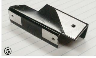
trapezoidal mask and hole on top (which will be oriented to the bottom) was only used in anticipation of securing the heatsink to the internal bulkhead. That wasn't found to be needed for heat dissipation, so that mask and hole can be omitted.
