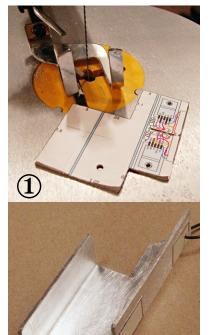
At left, the sheet metal is cut using a scroll saw with a metalblade. I used a paper template, pasted to the metal. Not sure if that was really better than just scribing the piece. The example here is the DIY replacement amp version but the original amp version is similar. The main difference is in adding a slot.<sup>1</sup>
