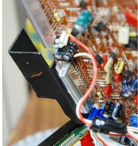
vious page (smaller arrow). At left is a closer view. It is formed from 0.0625" copper sheet metal. I obtained the material by splitting copper water pipe but that is the hard way. The heatsink should be painted flat black. Odd as it may seem to those not familiar, the paint improves emissivity. However, you should mask the surface which contacts the
