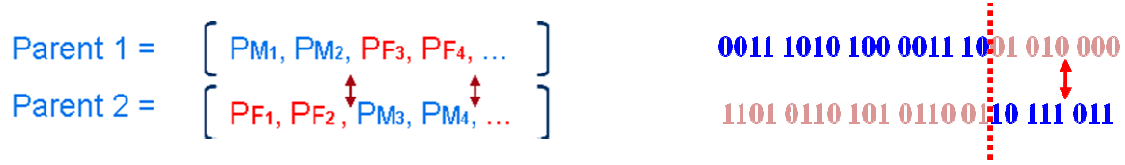
Figure 2-9: Crossover with only swapping in continuous and binary GAs
