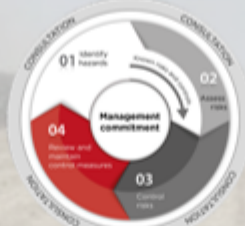
Figure 1. Risk management process Safe Work Australia
