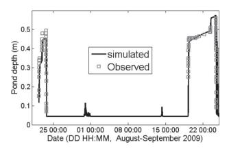
Figure 3. Observed and simulated pond's water heights during campaigns performed with the outlet closed (validation period).
