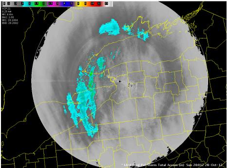
**Figure 4.** DP Storm Total Precipitation QPE from the Buffalo radar on October 28<sup>th</sup>, 2012 between 1004Z and 2002Z. The default 2.8 multiplier is used for dry snow and ice crystals. Note the melting layer discontinuity ring.
