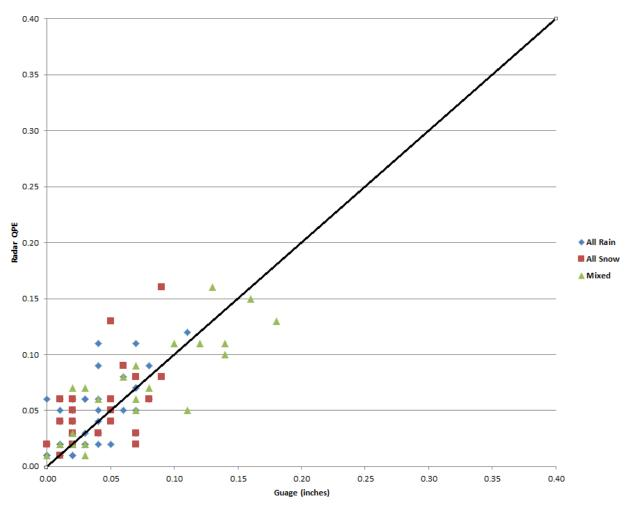
**Figure 3.** A scatterplot graph which compares DP QPE to gauge measured precipitation for 102 hourly cases with a 1.4 coefficient categorized by precipitation type at ground level.
