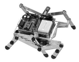
Fig 2: Optional Crawler kit connected to servo motors
