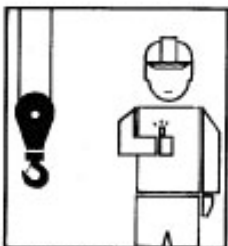
EXTEND BOOM- (Telescoping Booms) One Hand Signal. One fist in front of chest with thumb tapping chest.
