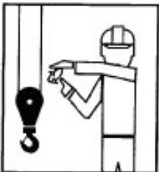
MOVE SLOWLY - One hand gives any motion signal; place other hand motionless in front of that hand. (Hoist slowly shown.)
