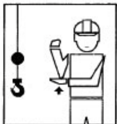
USE WHIPLINE- (Auxiliary Hoist) - Tap elbow with one hand; then use regular signals.
