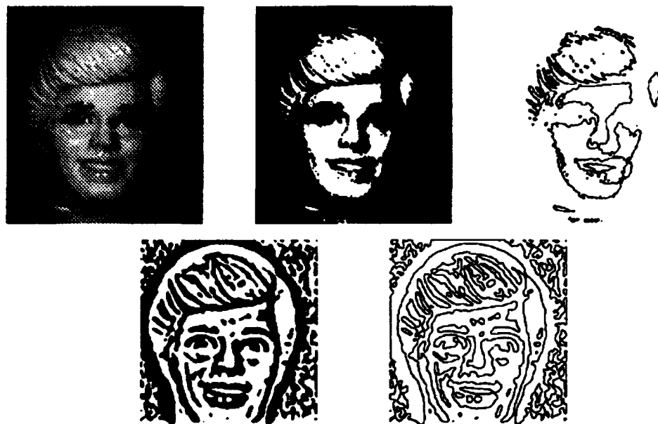
Figure 4.5: Top Row: A 'Ken' image represented by grey-levels, the same image followed by a threshold, the level-crossings of the thresholded image. The thresholded image shown in the center display is difficult to account for in computational terms, yet the original image was not lit in a way to create cast or attached shadows. Bottom Row: The sign-bits of the Laplacian of Gaussian operator applied to the original image, and its zero-crossings (step edges). Interpretability of the sign-bit image is considerably better than the interpretability of the zero-crossings.
