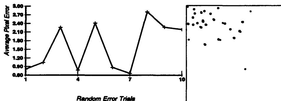
Figure 3.9: Random noise added to all image points, over all views, for 10 trials. Average pixel error fluctuates around 1.6 pixels. The result of re-projection on a typical trial with average error of 1.05 pixels, and maximal error of 5.41 pixels.
