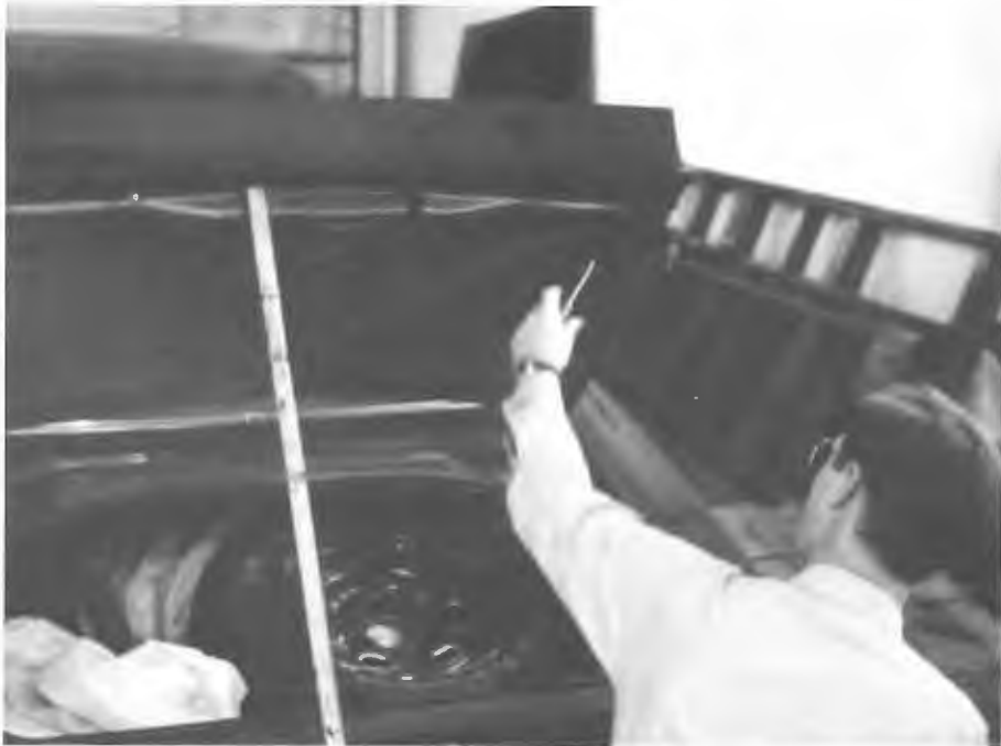
Ken of Emerald Detail demonstrating application of the rust proofing compound.
