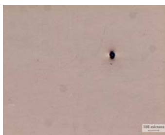
Figure 3-II-4: Polarized light and interferometric images of five defects caused by glass bubbles in Extruder Run 5 (Table 3-3).
