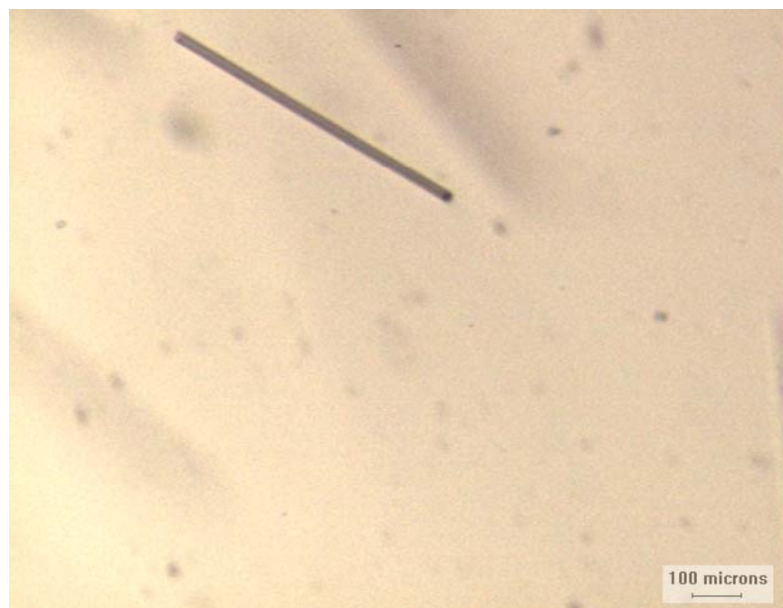
Figure 4-III-5: In-line image of glass fibers in low-density polyethylene melt obtained by the scanning particle monitor.
