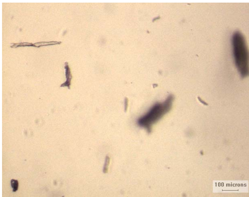
Figure 4-III-9: In-line image of wood pieces in low-density polyethylene melt obtained by the scanning particle monitor.
