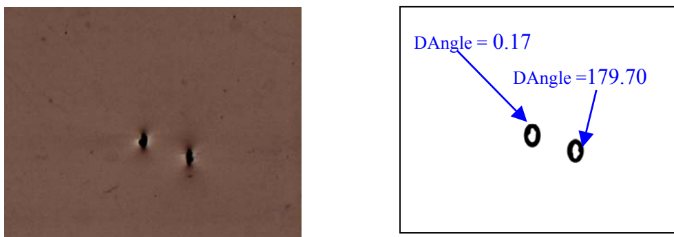
Figure 4-VI-4: (Left) Polarized light image of R24R30D06-1 and R24R30D06-2 defects caused by ceramic microspheres, (Right) Mask image of these defects. As you can see, these particles and defects are very similar. (The major axes of these defects are approximately parallel with the image vertical axis. The major axis of the top defect is slightly tilted to the right hand side of the vertical and the other is slightly tilted to its left hand side. This resulted in the huge difference in the DAngle values.)
