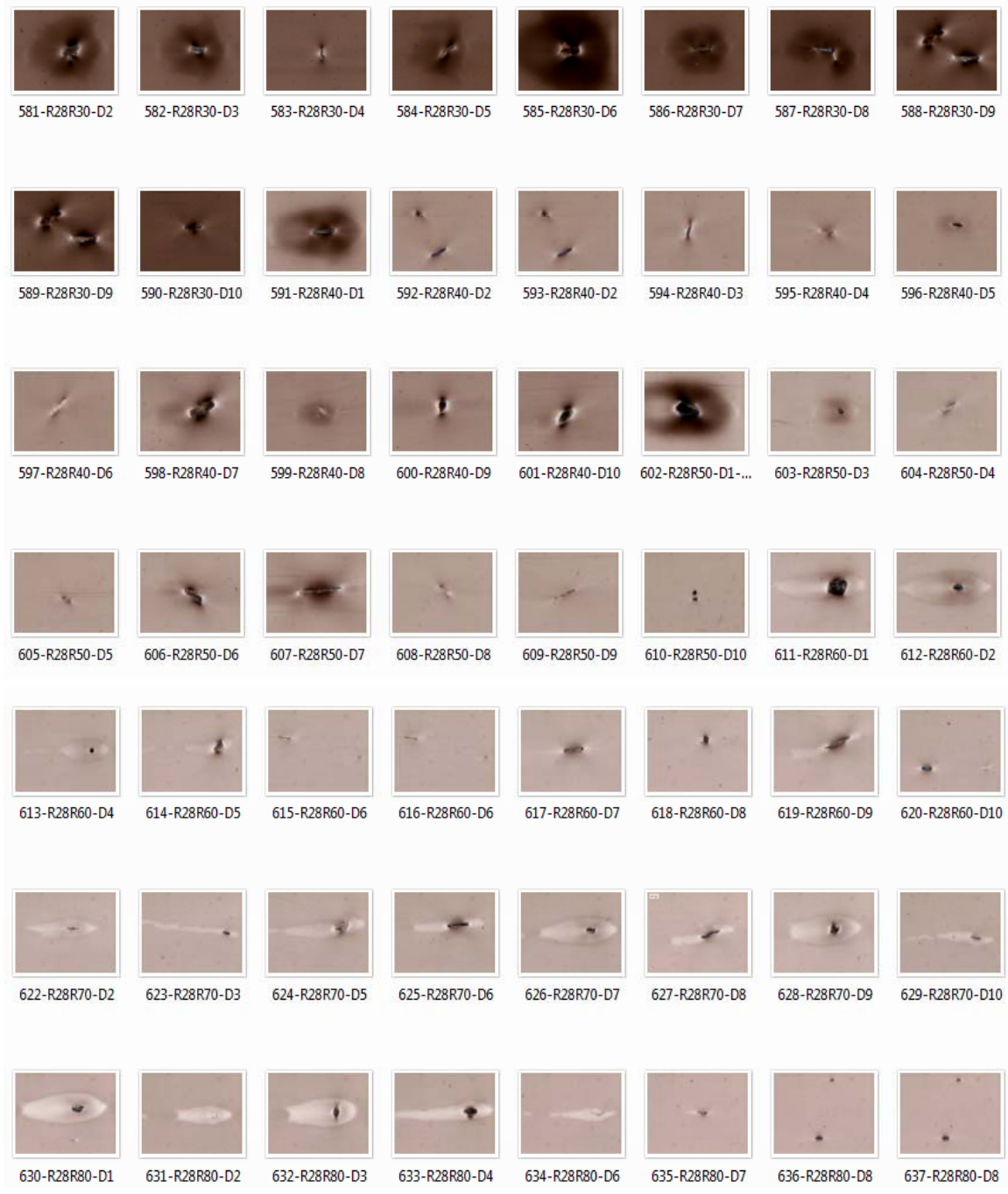
Figure 4-VII-1: Polarized light images of high average height and low average height defects caused by wood particles.
