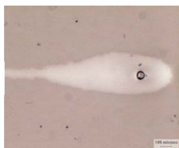
Figure 3-II-1: Polarized light and interferometric images of five defects caused by glass microspheres ( \sim 50 \mu\text{m} in diameter) in Extruder Run 2 (Table 3-3).
