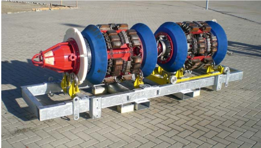
Figure 1: ROSEN's 26"/30" multi-diameter MFL tool with speed control
