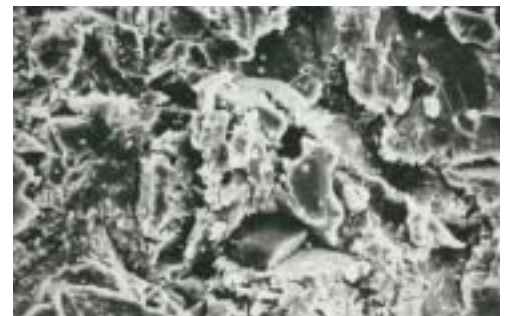
Metallic surface treated with MicroEtcher
