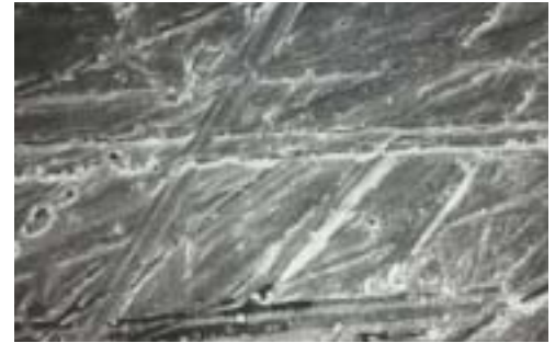
Metallic surface roughened with diamond bur
