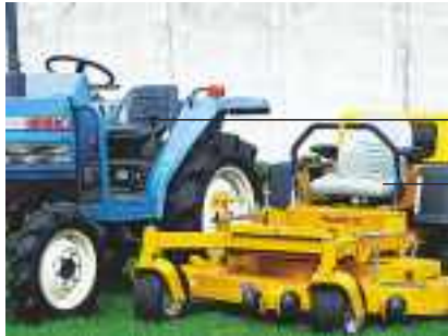
Hustler seat height of 660mm versus 1000mm on other typical machines. Some models of Hustler are even lower.
