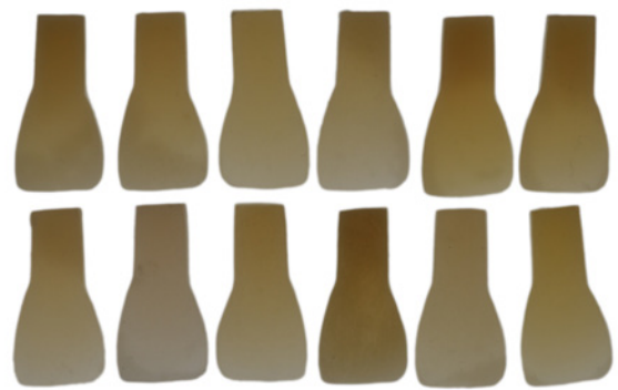
Figure 7. Different brands of composite resin, shown in the same thickness of A3 dentin, under indirect light. The differences between their opacity and light transmission are revealed.
