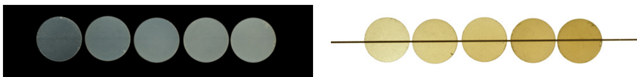
Figure 19. An effective composite enamel must increase its opalescence while increasing its thickness.
