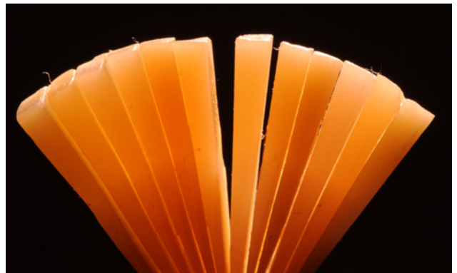
Figure 9. The same samples are shown under transmitted light. There are obvious differences in opacity, although all samples were calibrated to have the same thickness.
