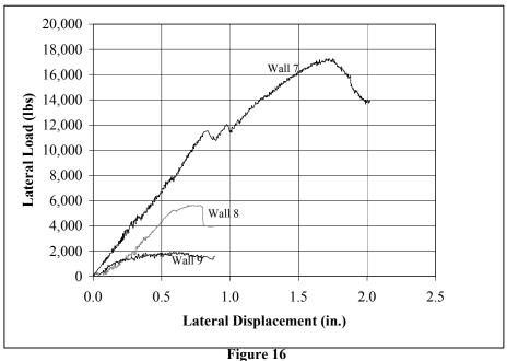
Force-Displacement Response for the Screen-Grid ICF Shear Wall Specimens (Wall 7, Wall 8, and Wall 9)
