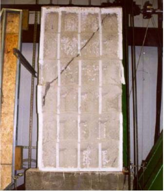
Figure 7 Failure Mechanism of Waffle No. 1 Wall Specimen
