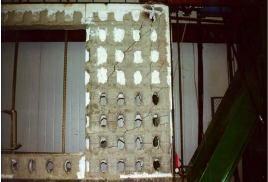
Figure 12 Failure Mechanism of Screen No. 2 Wall Specimen
