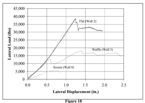
Force-Displacement Response for the 12ft x 8ft with Window Opening ICF Shear Wall Specimens (Wall 2, Wall 5, and Wall 8)
