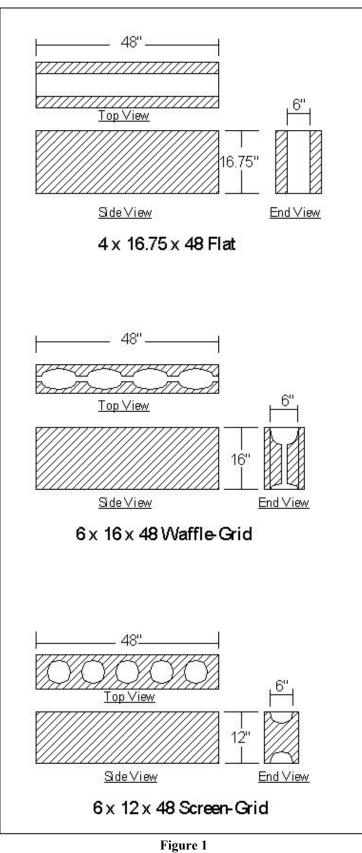
Diagrams and Dimensions of ICF Systems Used to Construct the Shear Wall Specimens
