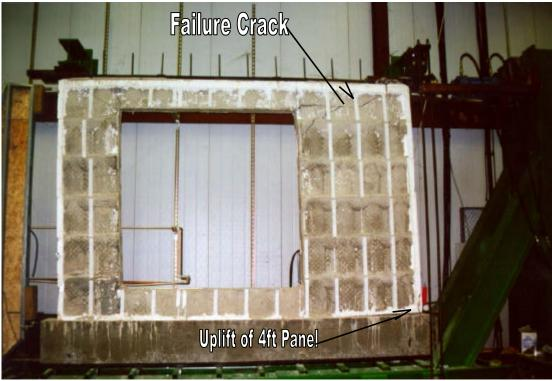
Figure 9 Failure Mechanism of Waffle No. 2 Wall Specimen
