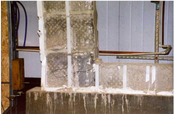
Figure 8 Typical Hairline Cracking at the Corner of the Window Opening (Waffle No. 2)
