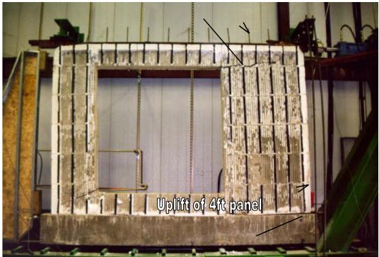
Figure 4 Failure Mechanism of Flat No. 2 Wall Specimen
