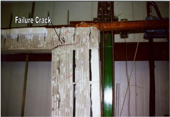
Figure 5 Failure Mechanism of Flat No. 3 Wall Specimen
