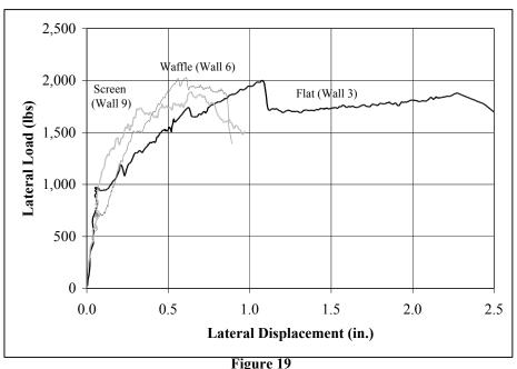
Force-Displacement Response for the 12ft x 8ft with Garage Opening ICF Shear Wall Specimens (Wall 3, Wall 6, and Wall 9)
