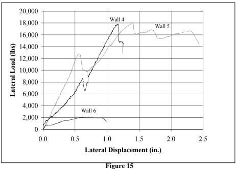
Force-Displacement Response for the Waffle-Grid ICF Shear Wall Specimens (Wall 4, Wall 5, and Wall 6)
