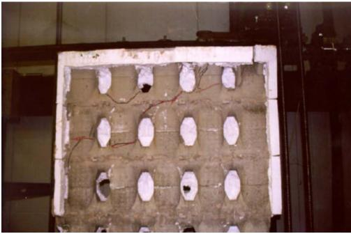
Figure 11 Failure Mechanism of Screen No. 1 Wall Specimen
