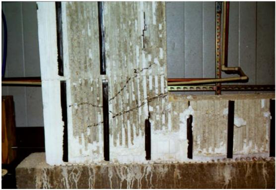
Figure 3 Typical Hairline Cracking at the Corners of the Window Opening
