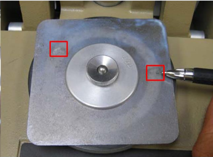
Poorly Adhered Coating (Mass Loss ~ 100mg/1000 cycles)
