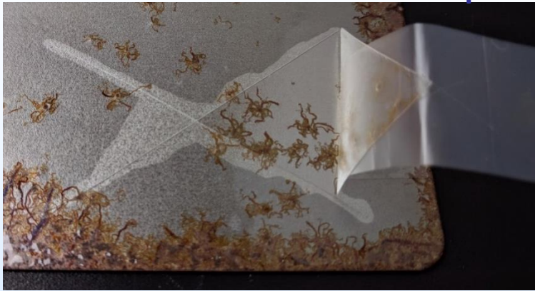
Knife adhesion test (ASTM D6677)
