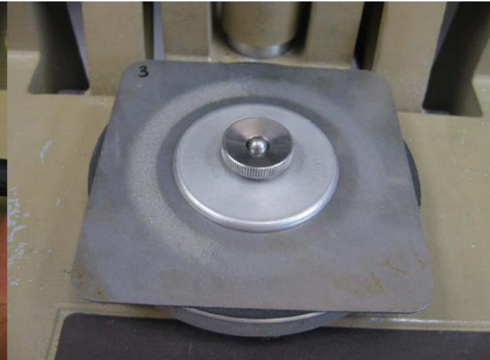
DragX™ Treatment (Mass Loss ~ 50mg/1000 cycles)
