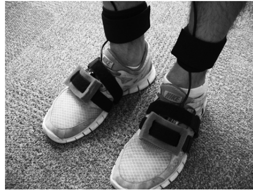
Fig. 1. MicroStrain 3DM-GX3-25 inertial/magnetic sensor module attached to the feet for position tracking
