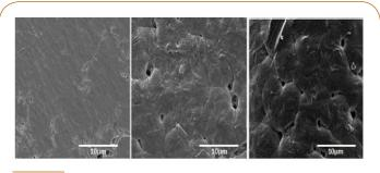
Figure 8 SEM pictures of a) nylon-1% b) nylon-3% c) nylon-6%.
