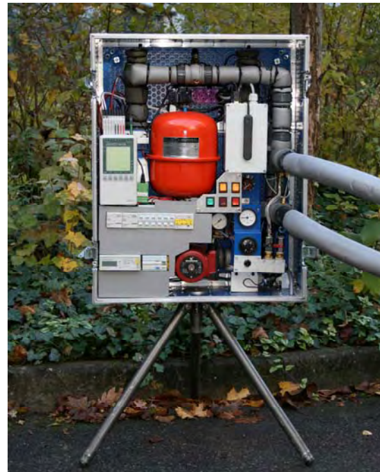
Figure 1: The in-situ thermal response test apparatus.
