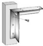
Flush mounted bracket mounts to the right side of the stud.
