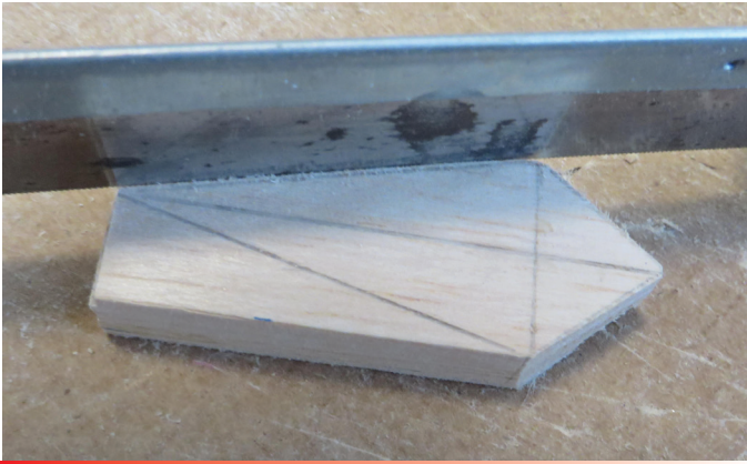
Figure 6: Use a fine tooth saw to cut along the lines you drew on the balsa when you started.
