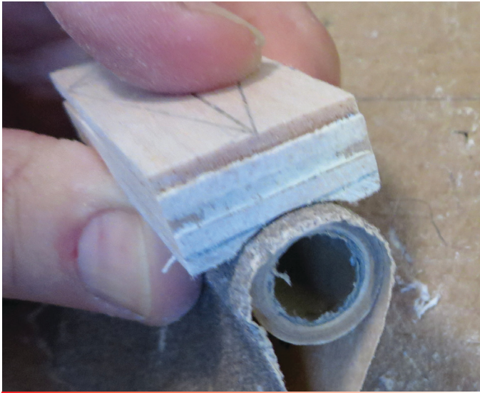
Figure 4: Use a spent engine casing to wrap your sand paper around to shape the bottom curvature of the balsa
