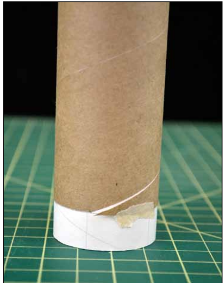
Figure 2 - Spiral-wound strips of paper can be used to create your own body tubes.
