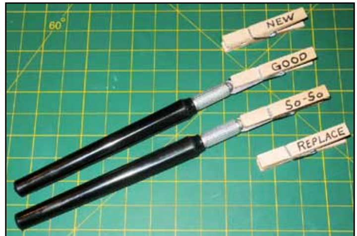
Picture 2: Keeping knives from rolling and letting you know the blade condition.
