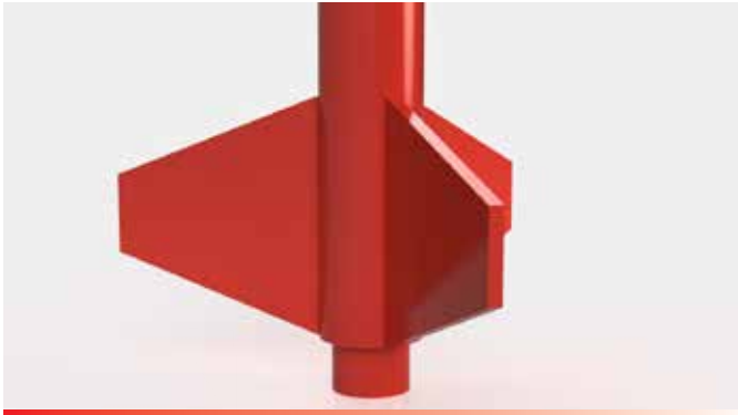
Figure 7: The cross section of this fin has a rectangular shape. You can tell by the sharp corners on the front and back edges.
