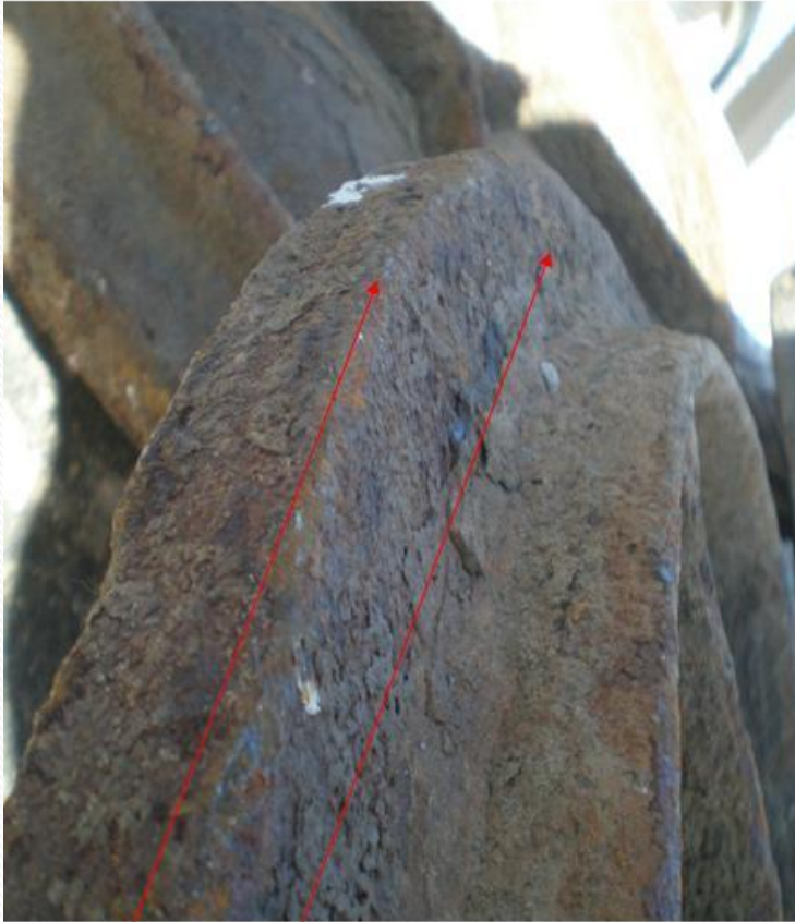
Rounded, tapered edge from rust and wear
