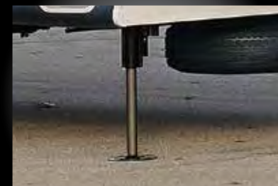
Wide stance hydraulic landing gear.
