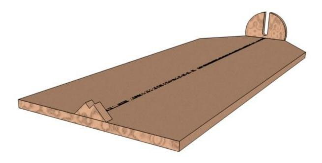
(In the drawing above, the notch may look higher than the center but it is not. The bottom of the notch and the center of the coupling are lined up at the same level, 1/2" above the top of the plywood)
