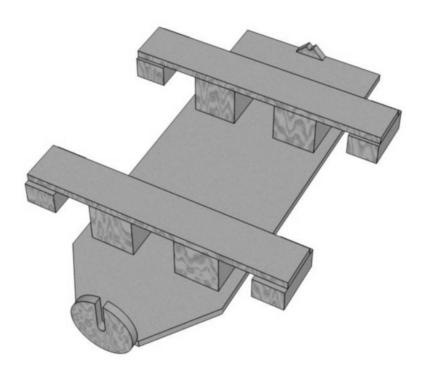
The flat piece of plywood represents the engine with transmission in plan view (from above).
