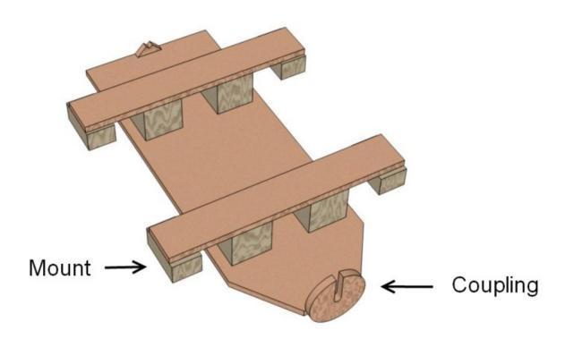
Coupling and mounts must be accurately fastened to the plywood template: coupling exactly on the centerline and mounts at the correct width, length and height.
