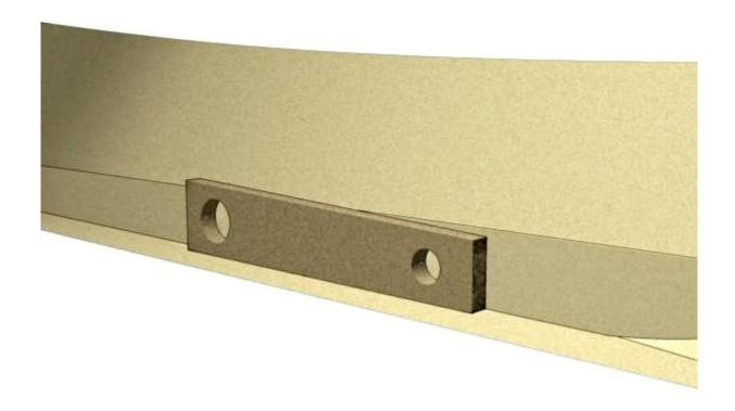
(In the drawing above, the engine beds are 2.50" wide. In length, they go from the frame in front of the engine to 12" behind the frame aft of the engine. The lightening holes are optional. The stringers height will be adjusted to the level of the top of the engine beds.)
