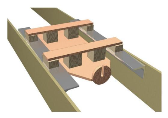
Above is a drawing of the template used to set up engine beds made of metal brackets between stringers.
