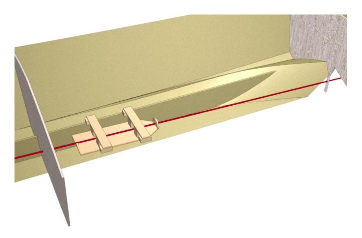
(This drawing shows one half of the ST21 hull with one stringer. This is a tunnel boat with a complex hull shape).
