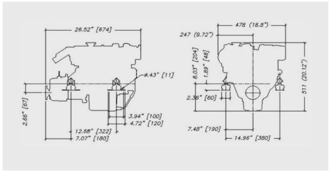
Note that the engine block shaft axis (crankshaft) and transmission shaft are different. Many engine dimensions are given relative to the crankshaft but our stern tube, prop shaft and engine beds must be lined up with the transmission axis. Because of the reduction gear, that axis is often offset a little below the engine block axis.
