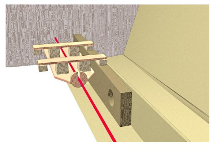
Do a final height adjustment and mark the outline of the beds on the stringers. Remove the template and epoxy weld the engine beds to the stringers then fiberglass. This done the same way than any other part of the framing: epoxy glued with fillets and taped seams.
