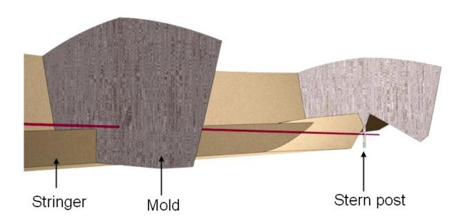
In our plans, we show reference points. Usually we show a point where the shaft axis traverse a mold or a frame forward of the engine and another on the stern post.
