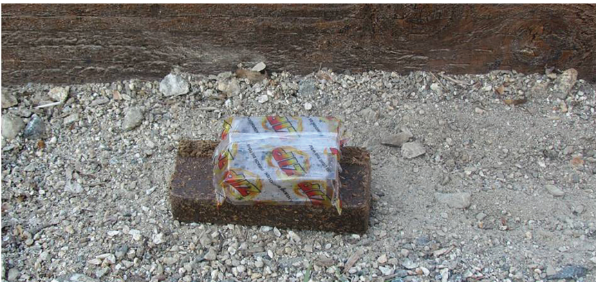
Hollywood Fire Devil: Device was a small fire log with a chemical booster placed on top. The combined flame height reached 14-18 inches, which started the underside of vehicles on fire. From Ed Nordskog's case files
