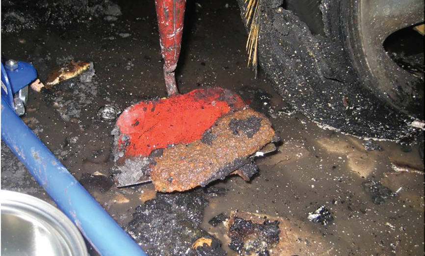
Burned Devices: Despite a large amount of fire damage at many scenes, investigators could easily pick out the burned remains of 49 out of 52 devices. From Ed Nordskog's case files, courtesy LAFD and LAPD.
