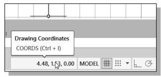
Note that the *coordinate display area* can also be used as a toggle switch; each left-mouse-click will toggle the coordinate display *on* or *off*.
