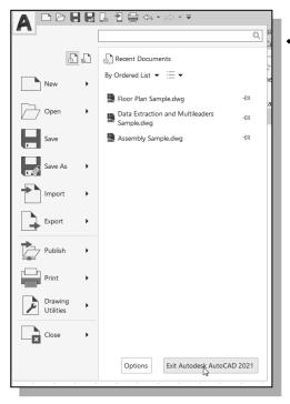
To exit AutoCAD 2021, select Exit AutoCAD in the Menu Bar or type QUIT at the command prompt. Note the command can also be activated with the quick-key combination of [Ctrl]+[Q].
