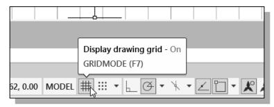
2. Move the cursor inside the graphics window, and estimate the distance in between the grid lines by watching the coordinates displayed at the bottom of the screen.
