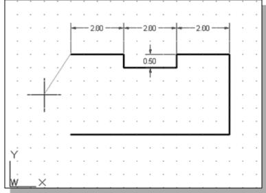
8. On your own, repeat the above steps and create the four additional line segments, using the dimensions as shown.
