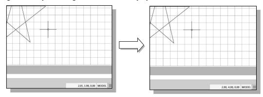
➤ The *GRID* option creates a pattern of lines that extends over an area on the screen. Using the grid is similar to placing a sheet of grid paper under a drawing. The grid helps you align objects and visualize the distance between them. The grid is not displayed in the plotted drawing. The default grid spacing, which means the distance in between two lines on the screen, is 0.5 inches. We can see that the sketched horizontal line in the sketch is about 4 inches long.
