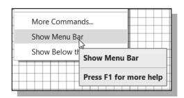
3. To switch on the **AutoCAD Coordinates Display**, use the *Customization option* at the bottom right corner.
