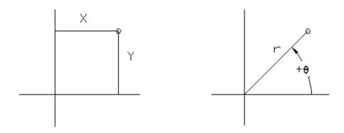
For planar geometry, the polar coordinate system is very useful for certain applications. In the polar coordinate system, points are defined in terms of a radial distance, r, from the origin and an angle  $\theta$  between the direction of r and the positive X axis. The default system for measuring angles in **AutoCAD 2021** defines positive angular values as counterclockwise from the positive X-axis.
