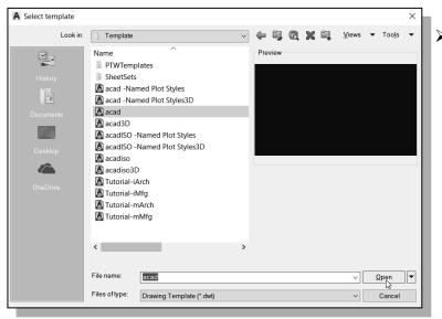
The dwt file type is the AutoCAD template file format. An AutoCAD template file contains pre-defined settings to reduce the amount of tedious repetitions.
