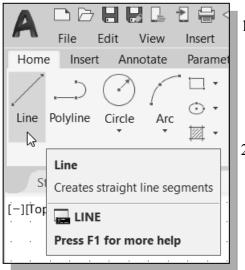
3. We will create a horizontal line by using the *relative rectangular* coordinates entry method, relative to the last point we specified:
