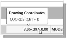
8. Left-click once on the *coordinates display area* to switch to a different coordinate display option. Click again to see the other option. Note the coordinates display has changed to show the length of the new line and its angle. Each click will change the display format of the cursor coordinates.
