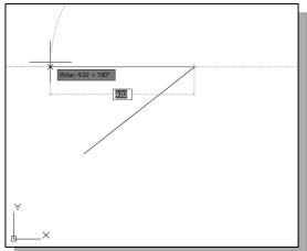
6. Repeat the above steps and complete the freehand sketch by adding three more lines (from *point 3* to *point 4*, *point 4* to *point 5*, and then connect to *point 5* back to *point 1*).
