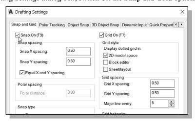
➤ On your own, exit the *Drafting Settings dialog box* and reset the status buttons so that only *GRID DISPLAY* and *SNAP MODE* are turned *ON* as shown.
