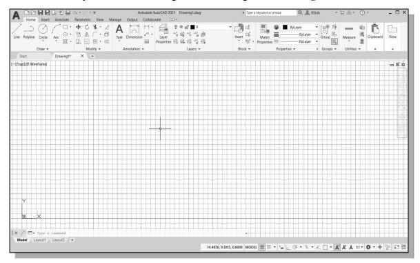
2. If necessary, click on the down-arrow in the *Quick Access* bar and select **Show Menu Bar** to display the **AutoCAD** *Menu Bar*. The *Menu Bar* provides access to all AutoCAD commands.
