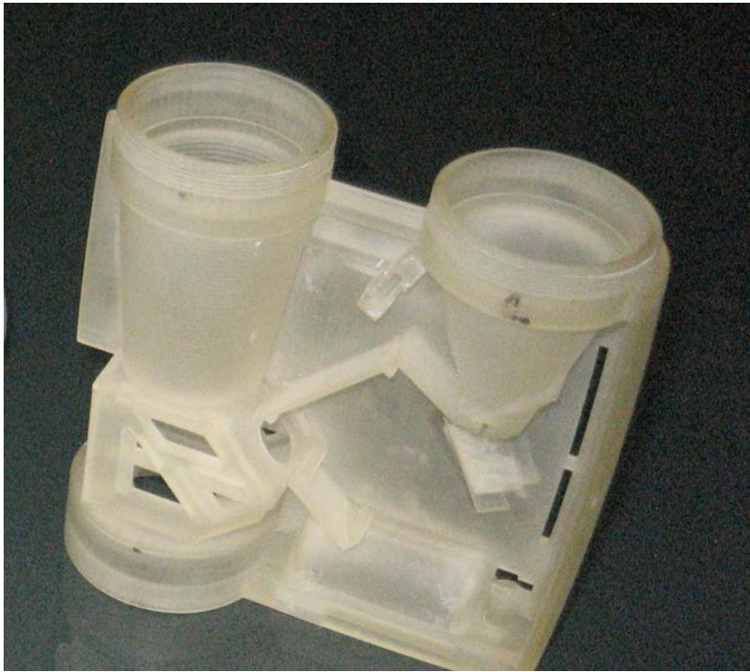
Rapid prototype of a laser rangefinder produced by stereolithography
