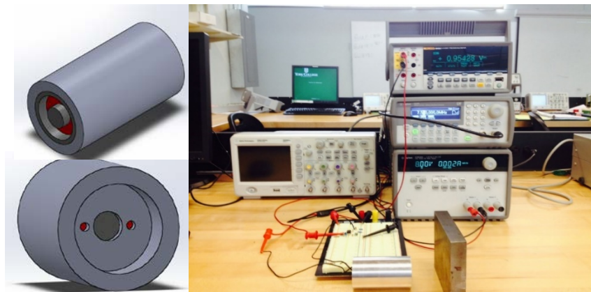
Figure 3: CAD of model of the inductive proximity sensor and the laboratory setup
