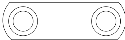
4 each 3/8 – 16 dual pilot rectangular nut
