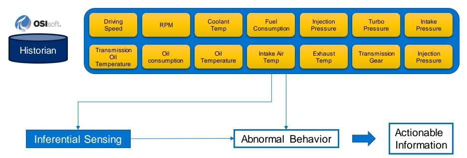
Predict key parameters (impractical to measure directly, but required for modelling) using the available data, based on engineering and physics
