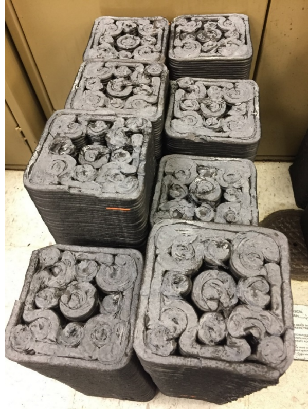
Figure 13: Set 4 showing the increased contact area between layers.
