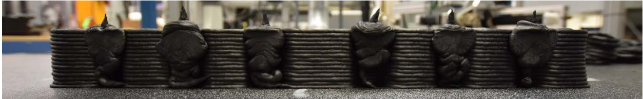
Figure 3: A print done to find the optimal hole size. Outer holes show the polymer didn't reach the base of the hole.
