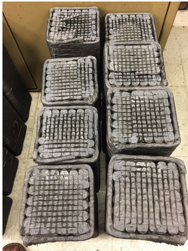
Figure 14: Set 1 with less contact area than set 4.
