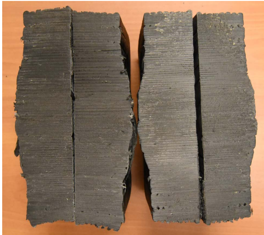
Figure 4: Two cross-sectioned parts with one central pin. The pin is not distinguishable because it is fully dense.
