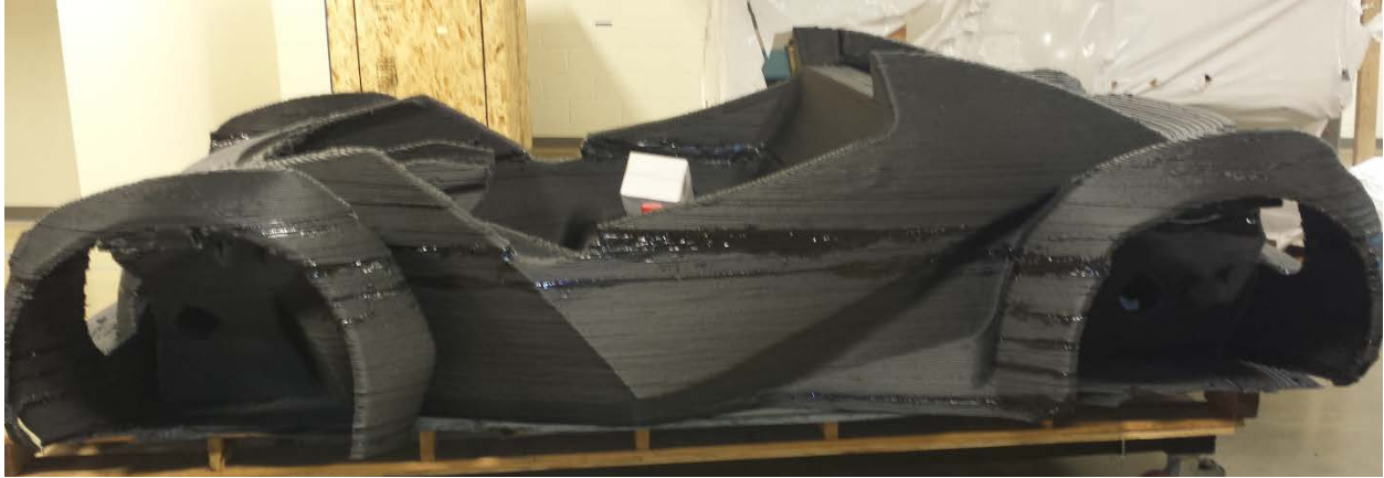
Figure 1: An early test print of the Strati that resulted in numerous delaminations that had to be glued together
