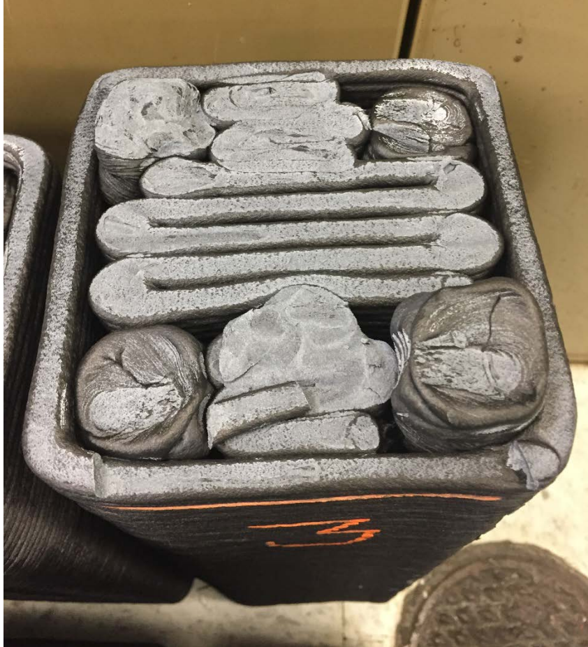
Figure 15: Fracture of a three-point bend sample. The bottom right pin illustrates a pull-out.
