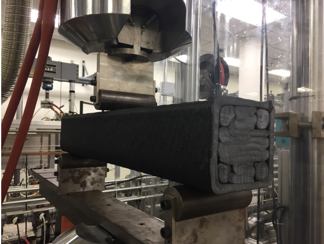
Figure 12: Three-point bending machine setup
