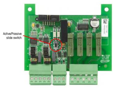
Figure A-41: COM2/Discrete I/O (Relay) Option Board
