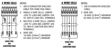
Figure A-31: Load Cell TerminationS
