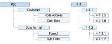
Figure 3-12: Setup Menu for DeviceNet
