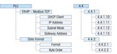
Figure 3-11: Setup Menu for Ethernet/IP and Modbus TCP
