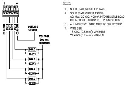
Figure A-48: Relay Outputs
