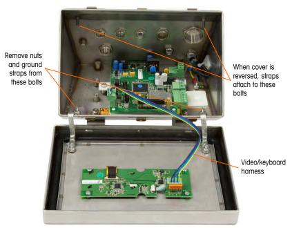
Figure A-20: Loosening the Ground Straps
