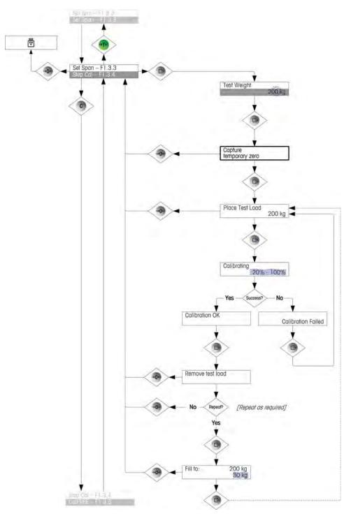
Figure 2-13: Step Calibration
