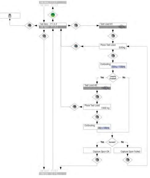
Figure 2-12: Span Calibration
