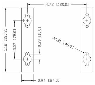
Figure A-22: Mounting Hole Pattern
