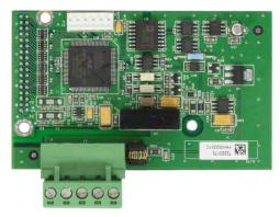
Figure A-49: Analog Output Option Board
