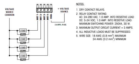
Figure A-45: Relay Outputs
