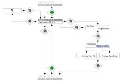
Figure 2-11: Zero Calibration
