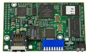
Figure A-59: Ethernet / IP Option Board
