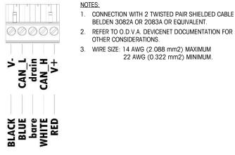
Figure A-54: DeviceNet Connector Wiring
