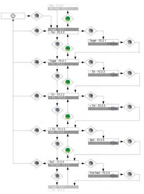
Figure 2-9: Target Setup Screens
