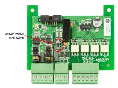
Figure A-46: COM2/Discrete I/O (Solid State) Option Board
