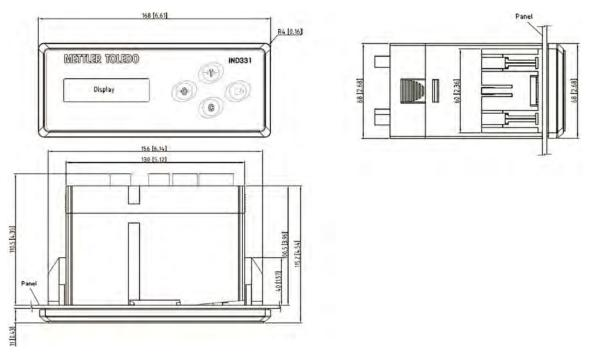
Figure 1-3: IND331 Panel Mount Enclosure Dimensions
