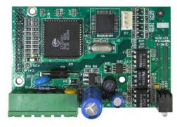
Figure A-53: DeviceNet Option Board
