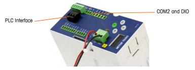
Figure A-38: Option Locations in the DIN, Panel-mount and J-Box Modules
