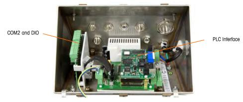
Figure A-39: Option Locations in the Harsh Enclosure
