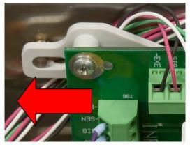
Figure A-32: Removing the Summing Board
