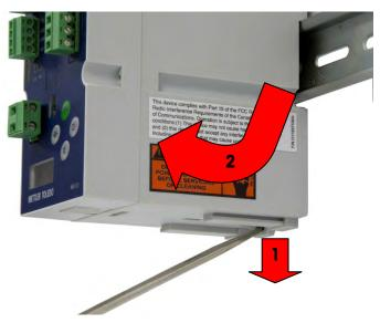
Figure A-7: Removing Module from DIN Rail
