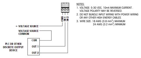
Figure A-44: Passive Input Connections
