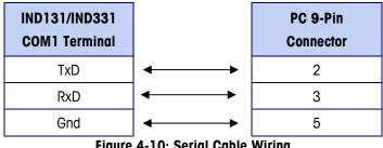
Figure 4-10: Serial Cable Wiring
