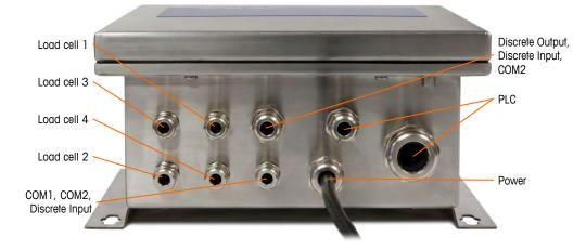
Figure A-25: J-Box Enclosure Gland Assignments
