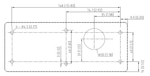
Figure 1-6: IND331 Panel Mount Drill Template
