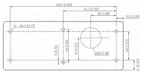
Figure A-8: Panel Mounting Template
