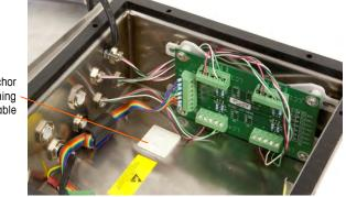
Figure A-36: Load Cell Wires Installed and Routed, Summing Board Mounted
