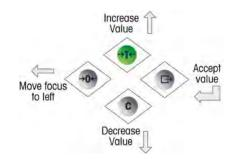
Figure 2-4: Key Functions When Viewing the Operator Menu
