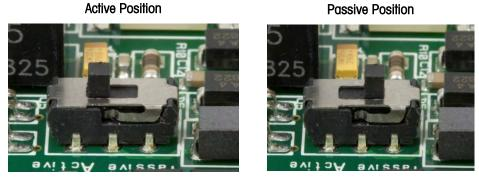
Figure A-47: Active/Passive Input Switch
