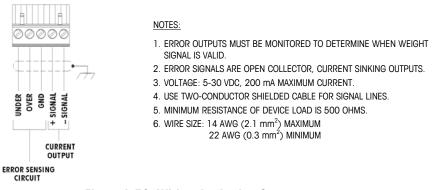
Figure A-50: Wiring the Analog Output
