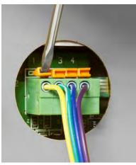
Figure A-15: Orange levers on display board connector
