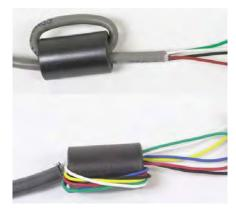
Figure A-23: Installing the Ferrite Core
