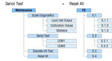
Figure 3-15: Maintenance Branch of Setup
