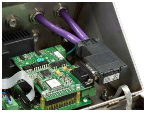
Figure A-57: Harsh Enclosure PROFIBUS Cable Routing
