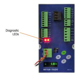
Figure 4-1: Diagnostic LEDs
