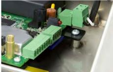
Figure 4-8: SD Memory Card Insertion, IND331 in Harsh Enclosure
