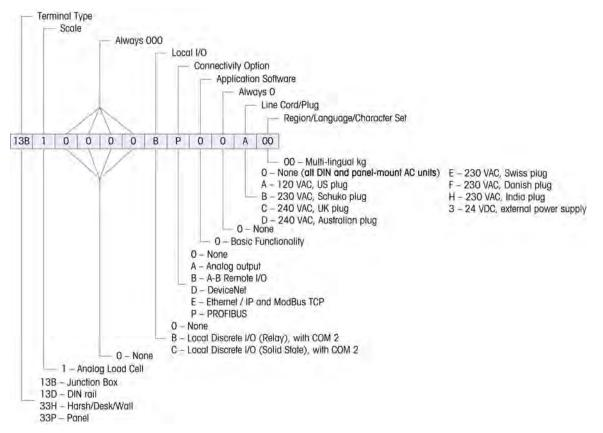
Figure 1-1: IND131/IND331 Model Identification Numbers
