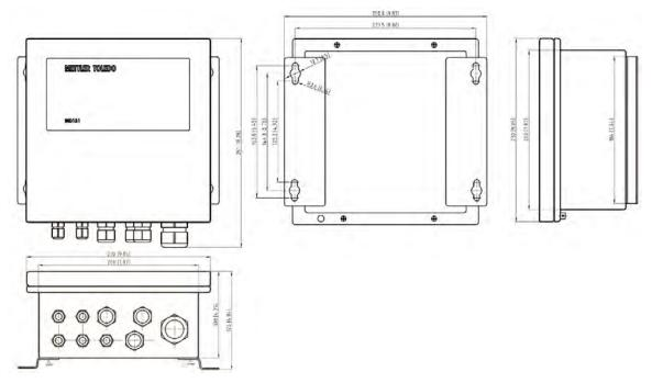
Figure 1-5: IND131 Junction Box Enclosure Dimensions
