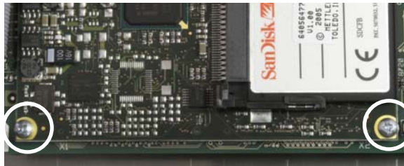
Figure 3-42: ETX Board Mounting Screws
