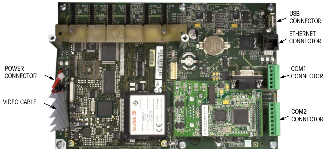
Figure 3-11: Main PCB Connections and Mounting Screws
