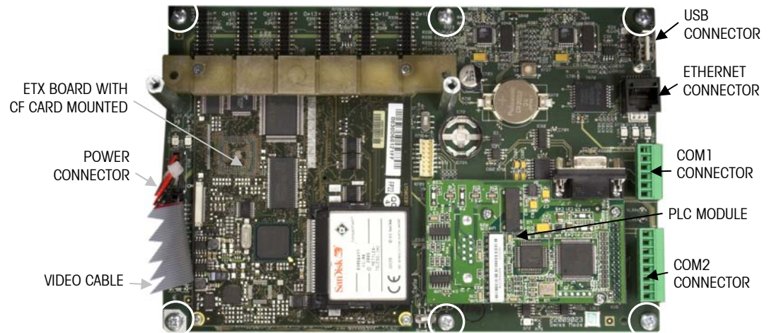
Figure 3-39: Main PCB Connections and Mounting Screws
