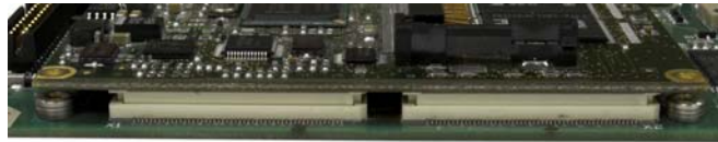
Figure 3-44: ETX Board Resting on Connectors
