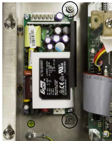
Figure 3-50: Power Supply, Disconnected
