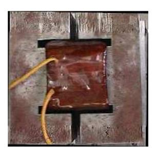
Figure 4.19: Left: Schematic drawing of the 1:100 scale model, Right: Photograph of the 1:100 model magnet with split iron pieces.
