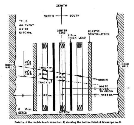
Figure A-3: An expanded view of a section of Telescope 2 in which an inelastic collision in rock of an upward moving neutrino was recorded. The black dots are the fired NFT's.
