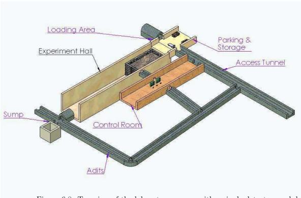
Figure 6.8: Top view of the laboratory cavern with a single detector module
