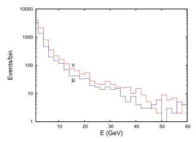
Figure 5.3: Number of events in GeV bins from 5 years' CC atmospheric muon neutrino interactions. The distributions both for the original neutrino and the generated muon, in the absence of oscillations, are shown.
