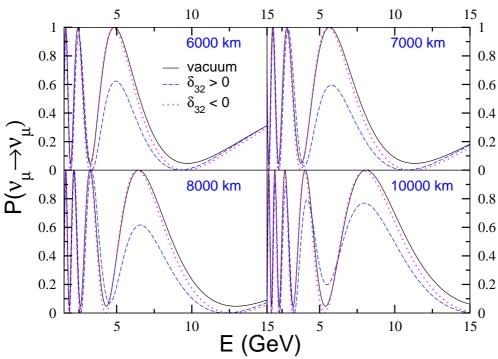
Figure 3.5: The muon survival probability in vacuum and in matter for both signs of  $\delta_{32}$  plotted against the neutrino energy for different values of baseline lengths, L (in km). The oscillation parameters used in all the plots are :  $\delta_{32} = 2 \times 10^{-3} eV^2$  and  $\sin^2 2\theta_{23} = 1$ .
