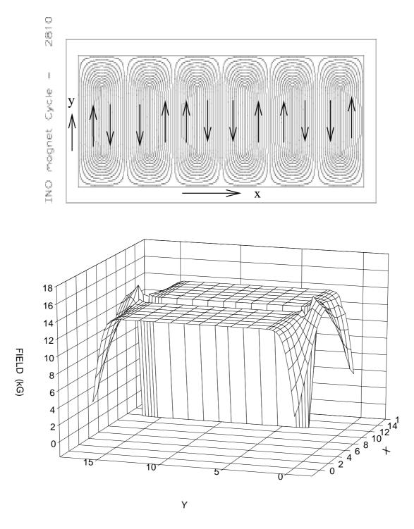
Figure 4.18: Top: Field lines in a horizontal plane of any of the iron plates, the arrows denote the field direction. Bottom: Magnetic field in a horizontal plane inside an iron plate.
