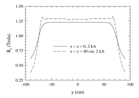
Figure 4.25: Top: Plot of magnetic field  $B_y$  vs y for x=z=0 thick(black) and for x=z=40 cm thin(red) for a current of 1000 amps. The origin is at the centre of the magnet. Bottom: same as in Top but for a current of 2000 amp.
