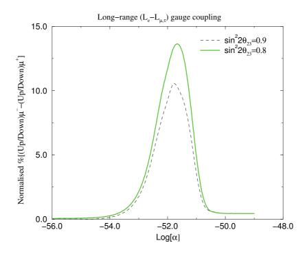
Figure 3.12: The neutrino-antineutrino asymmetry as a function of the  $L_e - L_{\mu,\tau}$  coupling  $\alpha \equiv g^2/4\pi$ . The plots show the percentage asymmetry for different  $\sin^2 2\theta_{23}$  and with  $\delta_{32} = 3 \times 10^{-2} eV^2$ .
