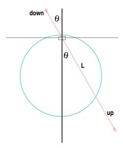
Figure 3.2: A schematic showing the up-coming and down-going neutrino directions and the path length L associated with the zenith angle  $\theta$ .
