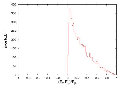
Figure 5.4: The figure shows the events distribution as a function of the fraction of neutrino energy carried by the muon. The data is a 5 years CC muon neutrino sample, without oscillations. Clearly most events fall in a region with small  $(E_{\nu} - E_{\mu})/E_{\nu}$ , indicating that the muon carries a substantial fraction of the neutrino energy in most events. Here  $E_{\nu}$  and  $E_{\mu}$  refer to the energies of the neutrino and muon respectively.
