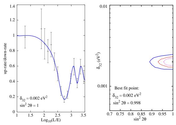
Figure 3.4: Left: The ratio of up to down muon events shown in Fig. 3.3 along with the statistical error bars plotted against  $\log_{10} L/E$ . The solid line is the best-fit curve. Right: The 68%, 90% and 99% CL contours obtained from the fits with the cross depicting the best-fit parameter values in  $\delta_{32}$  and  $\sin^2 2\theta_{23}$  parameter space.
