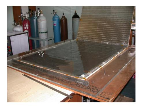
Figure 4.15: Photograph of 1  $\mathrm{m}^2$  RPC module with its pickup strips to be used for the ICAL prototype
