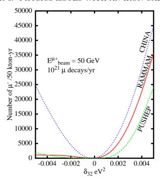
Figure 3.17: The same as Fig. 3.16, but for an upgraded neutrino factory configuration with a 50 kton-year exposure,  $10^{21}$  decays per year and a beam energy of 50 GeV.
