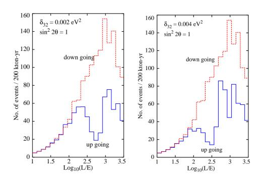
Figure 3.3: The number of up- (solid histogram) and down-going (broken histogram) muons (of either sign) in L/E bins are presented for two values of  $|\delta_{32}| = 0.002$ , 0.004 eV<sup>2</sup> for an exposure of 200 kton-years at ICAL.
