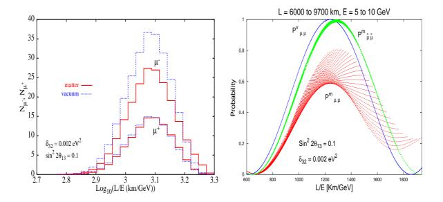
Figure 3.7: Left: The total event rate for muons and anti-muons in matter and in vacuum plotted against  $\log_{10}(L/E)$  for the restricted choice of L and E range. Right: The muon survival probability  $P^m_{\mu\mu}$  and the anti-muon survival probability  $P^m_{\bar{\mu}\bar{\mu}}$  in matter and in vacuum  $P_{\mu\mu}$  plotted against  $\log_{10}(L/E)$  for positive sign of  $\delta_{32}$ .
