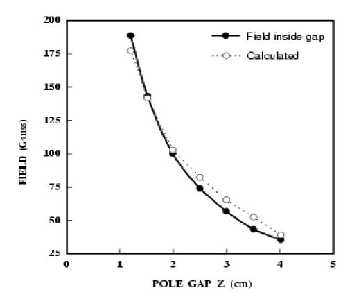
Figure 4.20: Calculated and measured field within the gap of the 1:100 prototypes.
