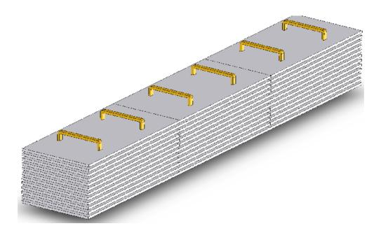
Figure 4.27: Layout of the coils (transverse) in Helmholtz-like pair design of the ICAL magnet.
