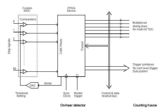
Figure 4.4: Proposed readout scheme for the ICAL detector.
