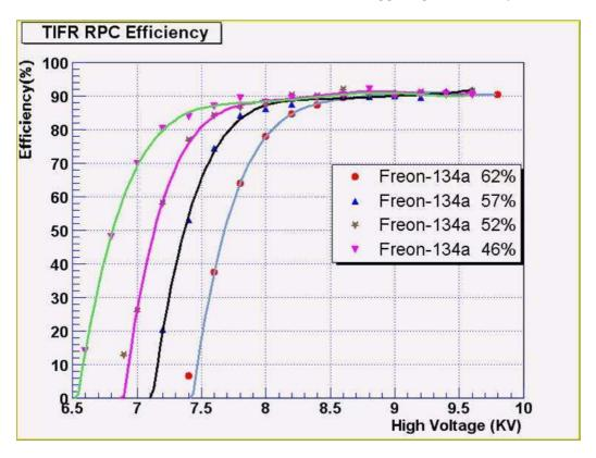
Figure 4.11: Efficiency plot of RPC as a function of applied voltage for various gas mixtures
