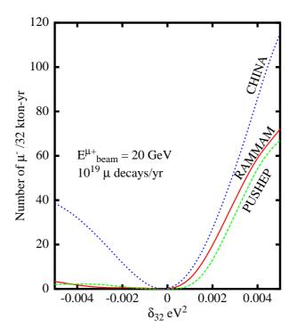
Figure 3.16: The number of wrong-sign muon events as a function of  $\delta_{32}$  for the three baselines from JHF, demonstrating the sign discriminating capability which arises as a result of matter effects. Event rates are computed for an entry-level configuration with a 32 kton-year exposure, beam energy of 20 GeV and  $10^{19}$  decays per year.
