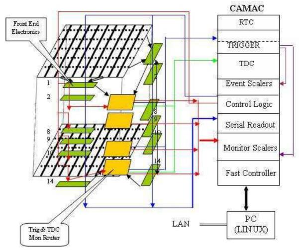
Figure 4.16: Schematic of the read-out electronics for the 1 m<sup>3</sup> prototype detector.
