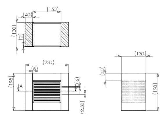
Figure 4.24: Standard 3-view of magnet with dimensions in cms (third angle projection).
