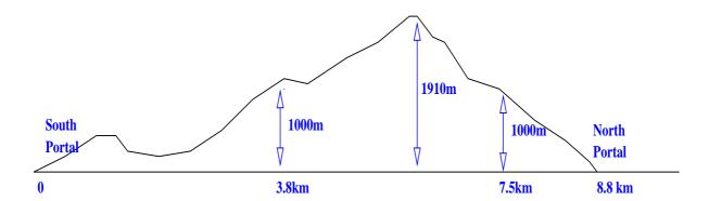
**Longitudinal Section above Rohtang Tunnel**
