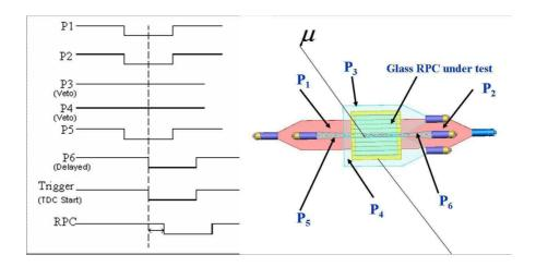
Figure 4.10: Schematic of cosmic ray telescope and muon trigger timing sequence.
