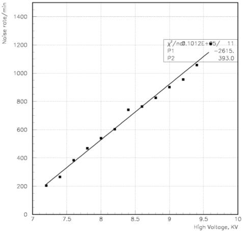
Figure 4.14: Typical noise rate plot of the RPC
