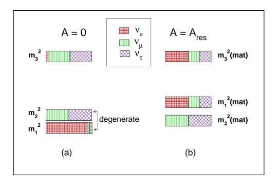
Figure 3.21: The flavours composition of mass eigenstates in vacuum (A = 0) and in matter at resonance  $(A = A_{res})$ . The vacuum parameters used are  $\sin^2 2\theta_{23} = 1.0$  and  $\sin^2 2\theta_{13} = 0.1$ .
