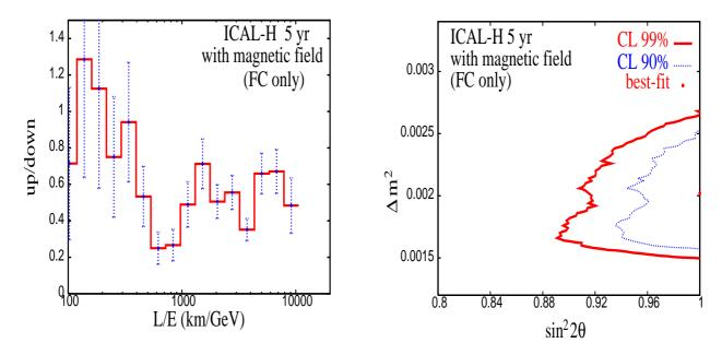
Figure 5.22: The (up/down) ratio as a function of (L/E) from a NUANCE sample of 5 years data with oscillation parameters  $\delta_{32}$ ,  $\theta_{23} = 2 \times 10^{-3} \text{ eV}^2$ , 45°. The best fit to this ratio gives an allowed oscillation parameter space shown on the right. Shown are the 90% CL and 99% CL regions and the best-fit value in the  $\delta_{32}$  eV<sup>2</sup>,  $\sin^2 2\theta_{23}$  parameter space.
