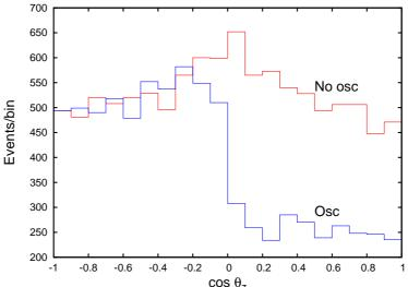
Figure 5.5: Zenith angle distribution of CC  $\nu_{\mu}$  events is shown by plotting the events rates per bin as a function of  $\cos\theta_z$  where  $\theta_z$  is the neutrino zenith angle. The bin size is 0.1. NUANCE labels "up-going" events as those with  $\cos\theta_z>0$ . These events are depleted when (2-flavour) oscillations are turned on, where oscillation parameters  $\delta_{32}, \theta_{23}=2\times 10^{-3}~{\rm eV^2}, 45^{\circ}$  have been used.
