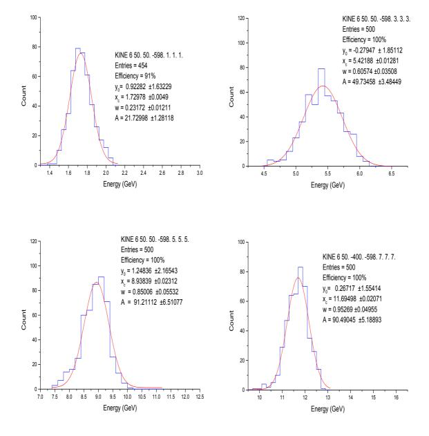
Figure 5.13: Distributions for the total energy for muons using fitting Algorithm I. The incident momenta are given in the KINE statement, which lists, in order, particle id (here muon), (x,y,z) in cm of the production point, and  $(p_x, p_y, p_z)$  in GeV.
