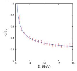
Figure 5.18: This figure shows the variation of the width of the gaussian distribution,  $\sigma$  as a function of the energy. Plotted is the ratio  $\sigma/E$  as a function of  $E_h$ , along with best fit curve.
