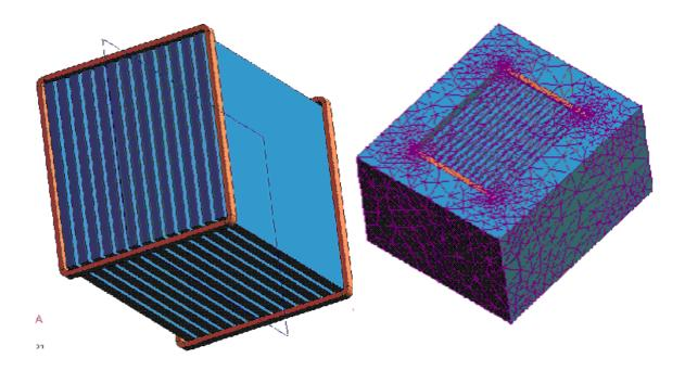
Figure 4.22: Left: Magnetic steel plates and copper coil, Right: a view of the magnet showing the mesh used in the calculation of magnetic field.
