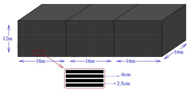
Figure 4.1: Schematic view of the iron calorimeter detector consisting of 140 layers of iron plates. Subdivision into three modules is also indicated.
