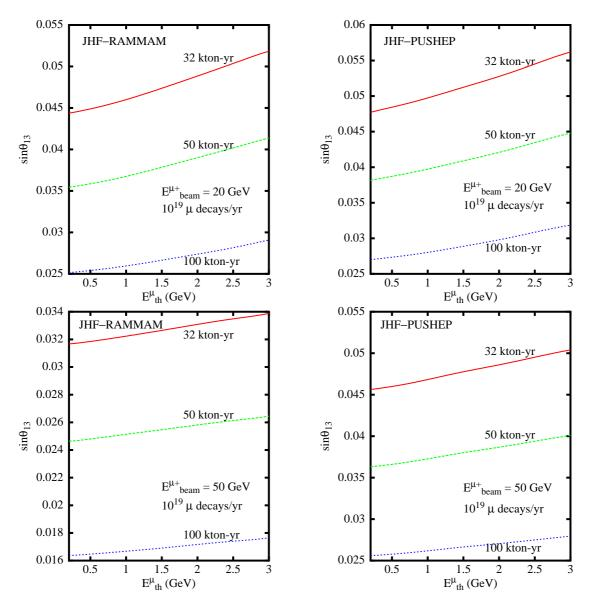
Figure 3.14: The  $\sin \theta_{13}$  reach for detector exposures of 32 kton-year, 50 kton-year and 100 kton-year for an entry-level neutrino factory configuration with  $E_{\mu}^{beam}=20$  GeV for the JHF-Rammam and the JHF-PUSHEP baseline. The lower panels show the change in reach if the storage muon energy is increased to 50 GeV, keeping the number of decays per year the same, i.e,  $10^{19}/\text{year}$ ; there is substantial improvement in the reach in the case of the JHF-Rammam baseline.
