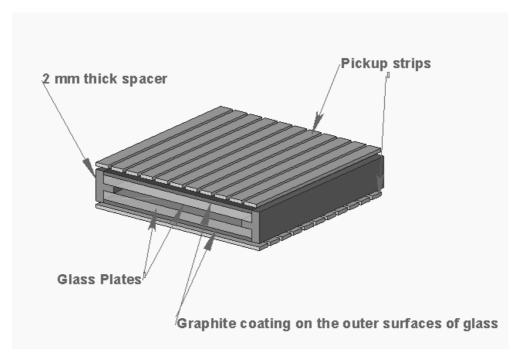
Figure 4.3: Sketch of a typical glass RPC unit.
