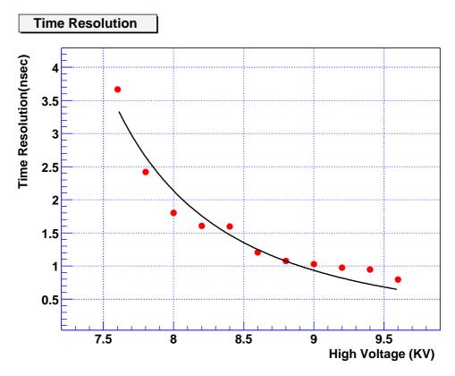
Figure 4.12: Typical timing resolution  $(\sigma)$  of an RPC as a function of applied voltage.
