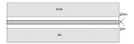
Figure 5.1: View of a unit cell of the simulated ICAL detector. The outermost layers are 3 cm of iron, with the sensitive detector (of gas, glass, G10 and copper from the centre out) symmetrically placed in a central 2.5 cm air gap. The detector is simulated as 140 unit cells, with top and bottom edge layers of 3 cm iron each.
