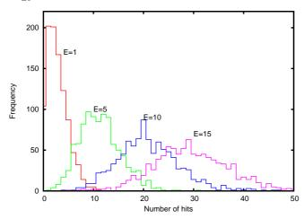
Figure 5.16: The frequency distribution of hits for fixed pion energies of  $E_h = 1, 5, 10, 15$  GeV, with 1000 random events per sample.
