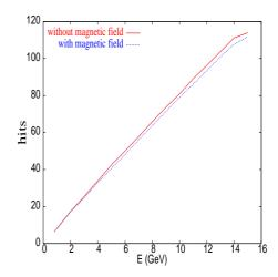
Figure 5.12: The variations of effective path-length (left) and number of hits (right) with energy for fixed  $\theta$  (= 40°) in ICAL-H for muons (without and with a magnetic field of 1 T in the z direction).
