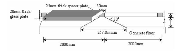
Figure A-3: Bearing width of the concrete floor.
