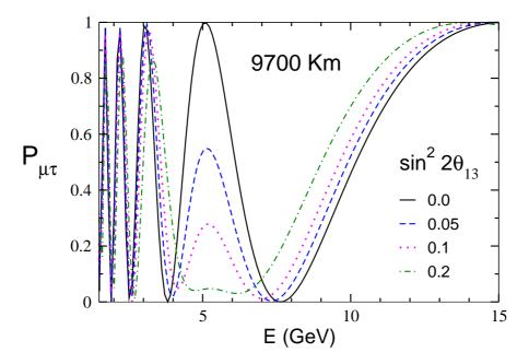
Figure 3.22:  $P_{\mu\tau}$  plotted against the neutrino energy, E(in GeV) for different values of  $\theta_{13}$ . We have used  $\delta_{31} = 0.002 \text{ eV}^2$ .
