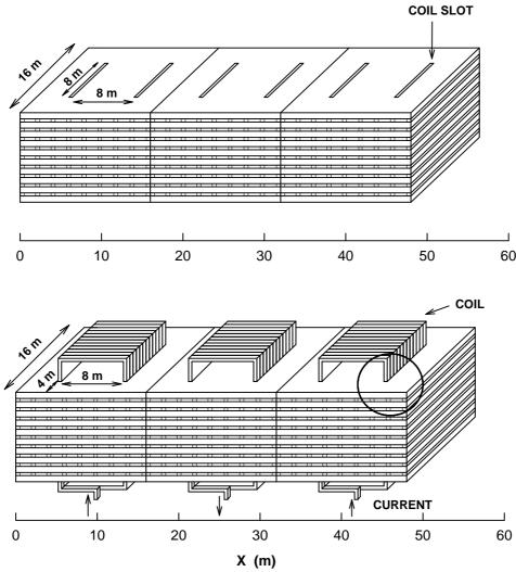
Figure 4.17: Top: ICAL magnet showing the coil slots and the iron plate arrangement. Bottom: magnet with the coil inserted.
