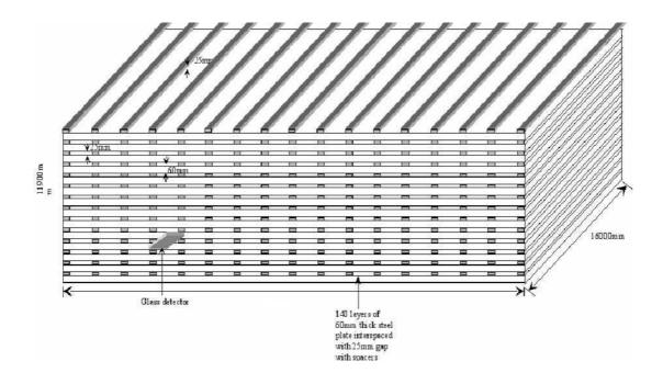
Figure A-4: Schematic view of ICAL including structural supports.
