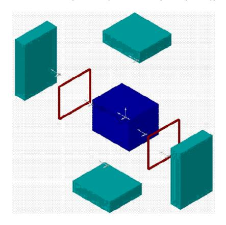
Figure 4.23: Exploded view of magnet (shaded view) parts. Shown in green is the yoke, in purple the magnetised steel plates and in red are the copper coils.
