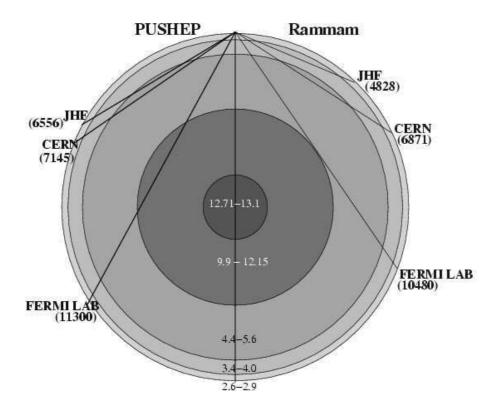
Figure 3.13: Base lengths(kms) from the proposed neutrino factories to the two proposed INO sites in India: Left half shows the base lengths to the site at PUSHEP whereas the right-half shows the base lengths to the site at Rammam. The densities of the layers that the neutrinos pass through are also indicated.
