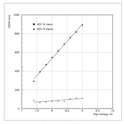
Figure 4.13: Typical mean charge (in arb. units) as a function of applied HV across an RPC
