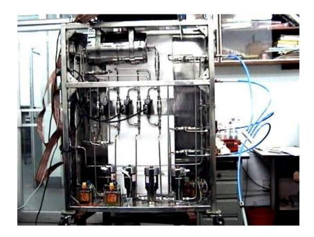
Figure 4.8: A photograph of the gas mixing unit being tested at SINP.
