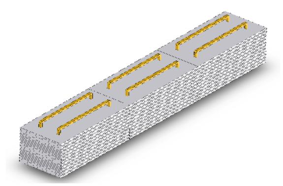
Figure 4.26: Layout of the coils (longitudinal) in Helmholtz-like pair design of the ICAL magnet.
