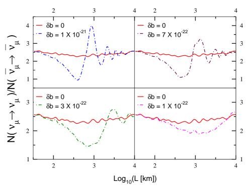
Figure 3.10: The ratio of total (up+down) muon to anti-muon events plotted against  $\log_{10}(L)$  for different values of  $\delta b$  (in GeV). The oscillation parameters used in all the plots  $\delta_{32} = 2 \times 10^{-3} eV^2$  and  $\sin^2 2\theta_{23} = 1$ .
