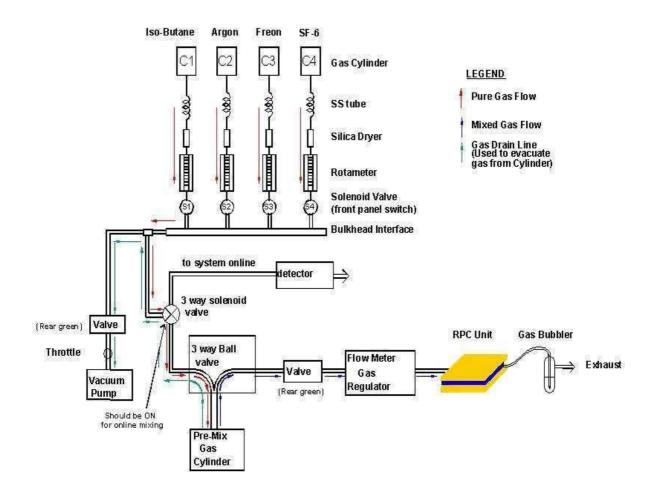
Figure 4.6: Schematic view of the gas mixing unit and control system at TIFR.
