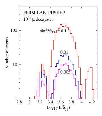
Figure 3.15: The number of wrong-sign muon events as a function of  $E_{\nu}/\delta_{32}$  (GeV/eV<sup>2</sup>) for the FERMILAB–PUSHEP baseline. The dip to the left of the distribution is due to a minimum of the oscillation probability.
