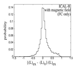
Figure 5.19: The energy E (left) and path length L (right) resolution functions for the sample of fully and partially contained (FC+PC) events. Here  $E_{ex}$  and  $L_{ex}$  refer to the reconstructed energy and path length respectively while  $E_{\nu}$  and  $L_{\nu}$  are those of the initial neutrino.
