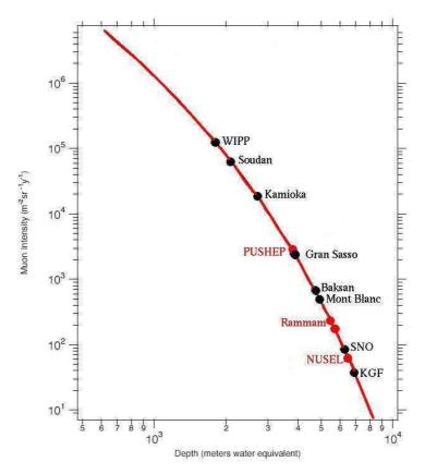
Figure 6.5: Atmospheric muon background as a function of depth. The best locations for INO correspond to backgrounds as in Gran Sasso or better.
