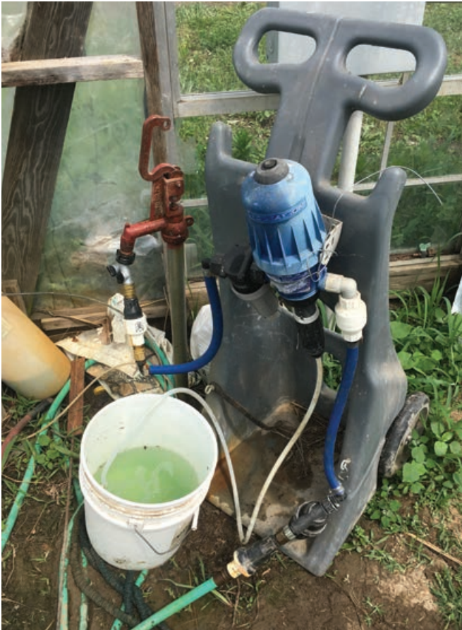
An example of a fertilizer application system that has been integrated with a drip irrigation system that is commonly used in high tunnels.
