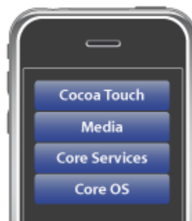
Figure 2-17: The four platform software layers of the iPhone OS (from [20])
