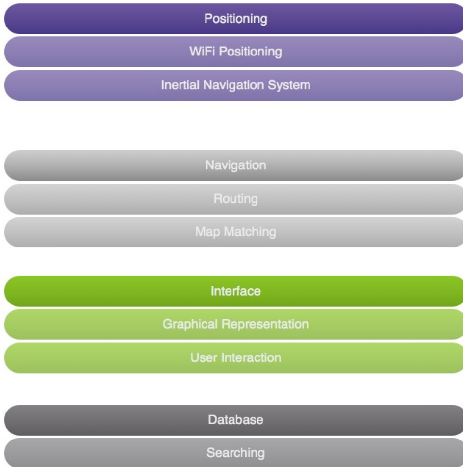
Figure 6-1: Application Software General Functional Blocks
