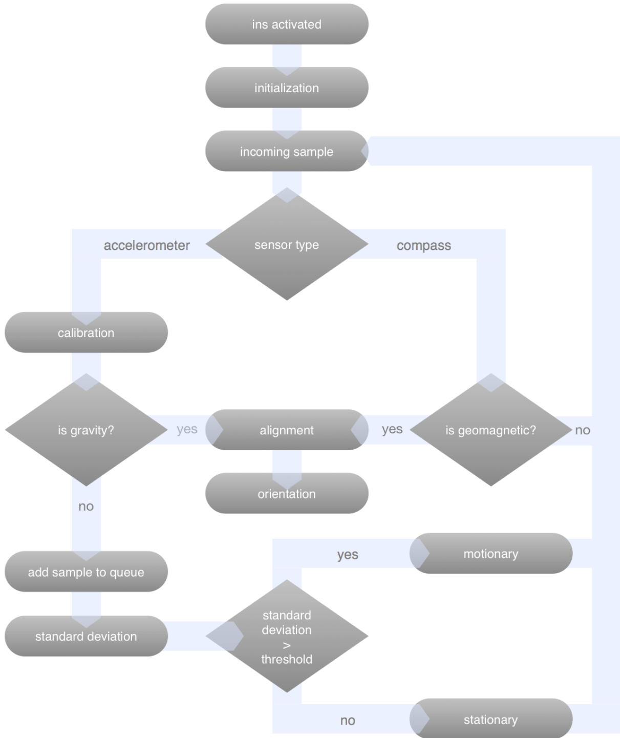
Figure 6-5: Inertial Navigation System Software Flowchart
