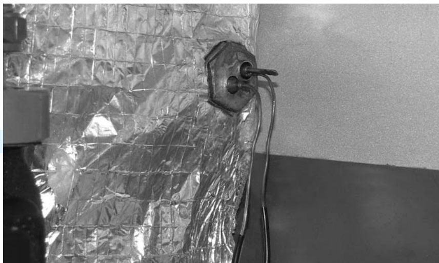
Figure 9-3: Thermostat phial position
