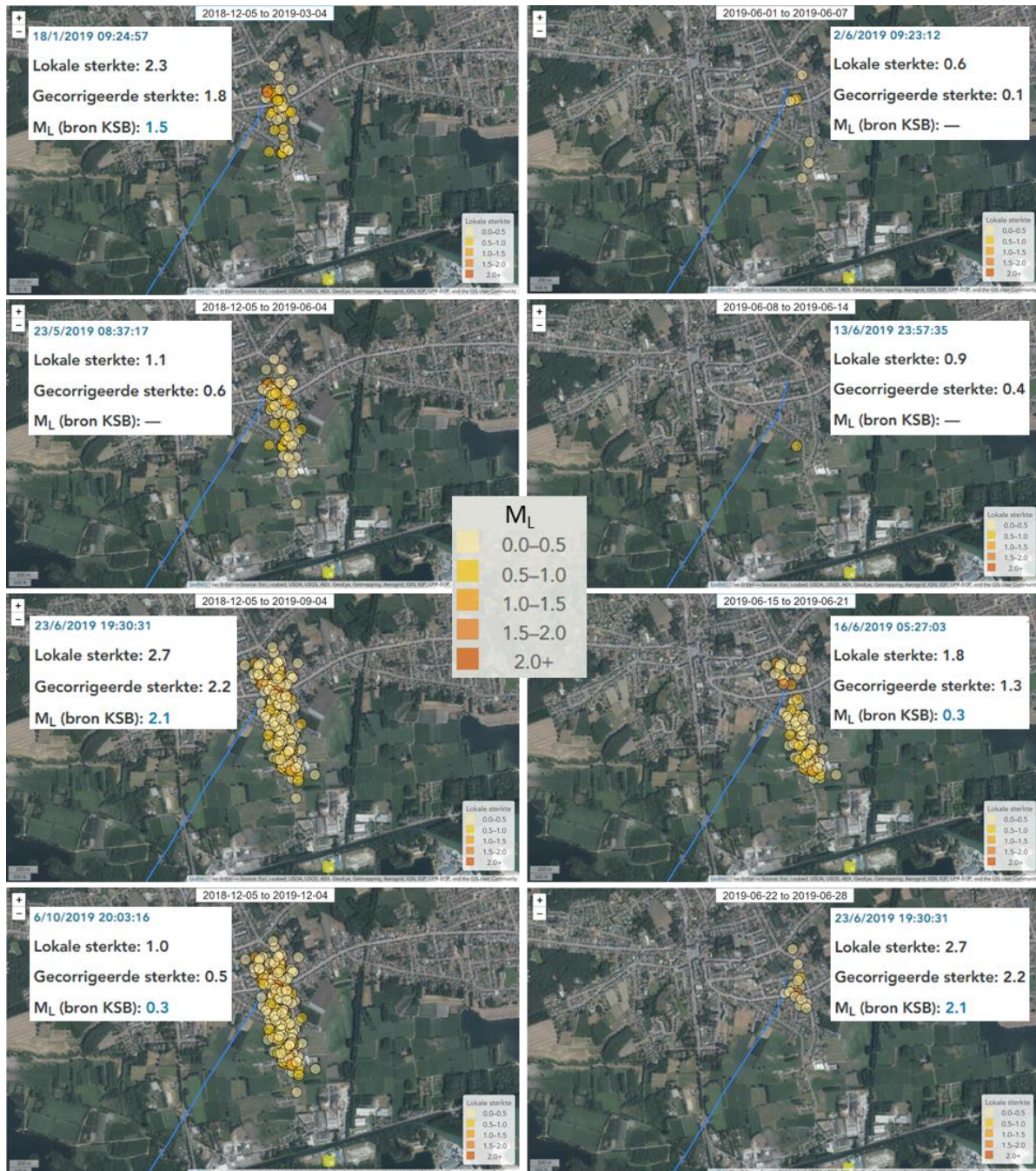
Figure 7-5 Development of seismicity (yellow-orange circles coloured according to magnitude, see legend) around production well MOL-GT-02 (blue line in NE direction) plot on a satellite image of the area. Text boxes indicate maximum magnitudes of seismic events for successive periods in time. Seismic station close to the well site is also indicated (yellow square). Left figures: Cumulative number of seismic events between 5 December 2018 and 4 December 2019 (1 year, each figure shows additional seismic events for a 3 month period). Right figures: Weekly occurrence of seismic events in June 2019 that led to the maximum M_L 2.1 on 23 June 2019, following an accidental power cut on the local electricity grid. Source: VITO (2020) 45 .
