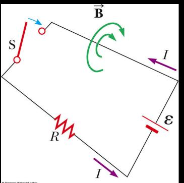
When the switch is closed, the battery (source emf) starts pushing electrons around the circuit.
