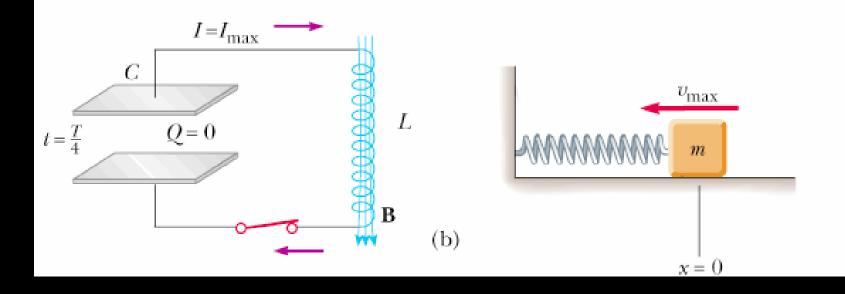
The current continues to flow and now starts to charge the capacitor again, this time with the opposite polarity.
