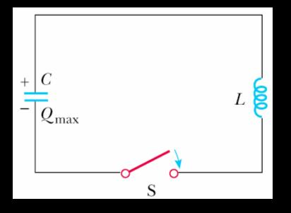
Provide a transfer of energy between the capacitor and the inductor.
