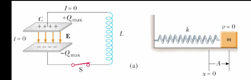
At the same time, the current increases the stored energy in the magnetic field of the inductor.
