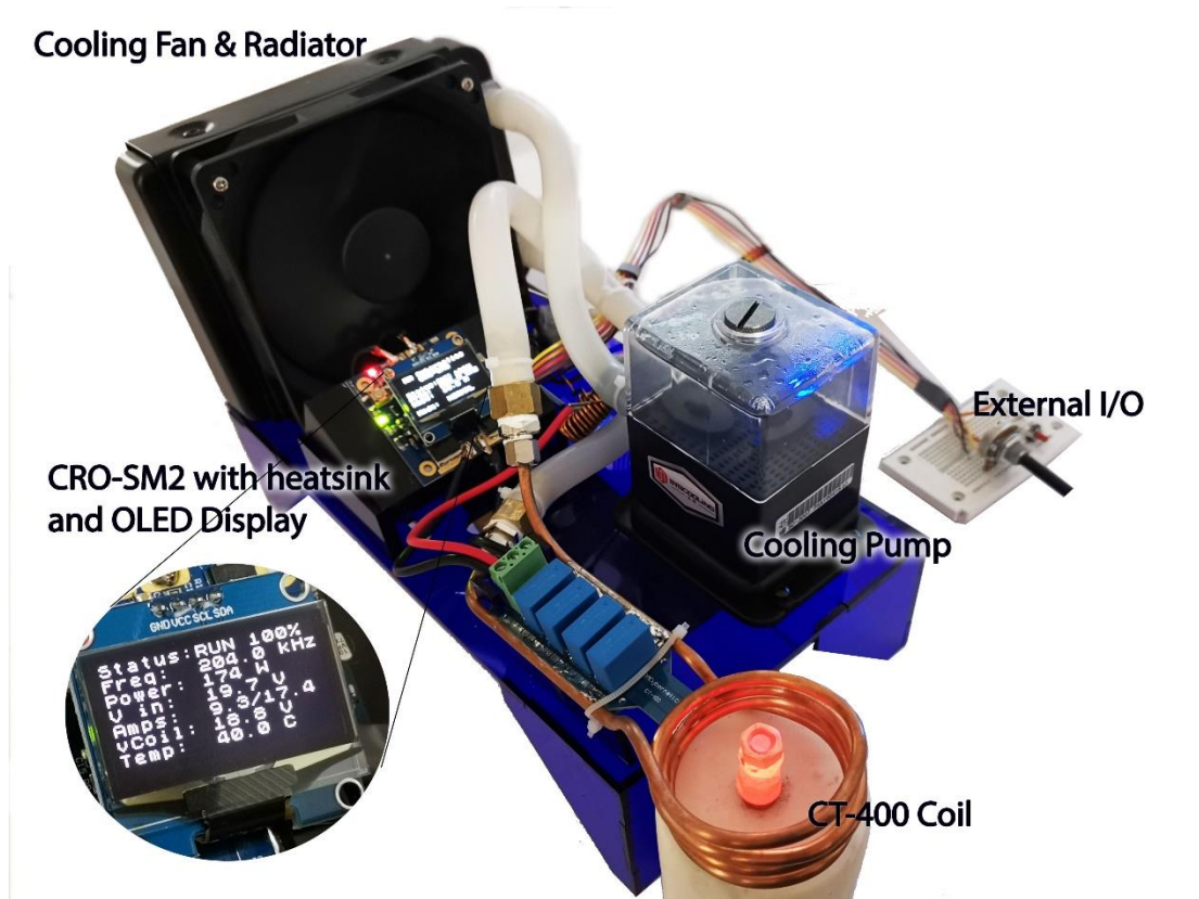
Figure 2: Example Water Cooled Induction Heater Setup
