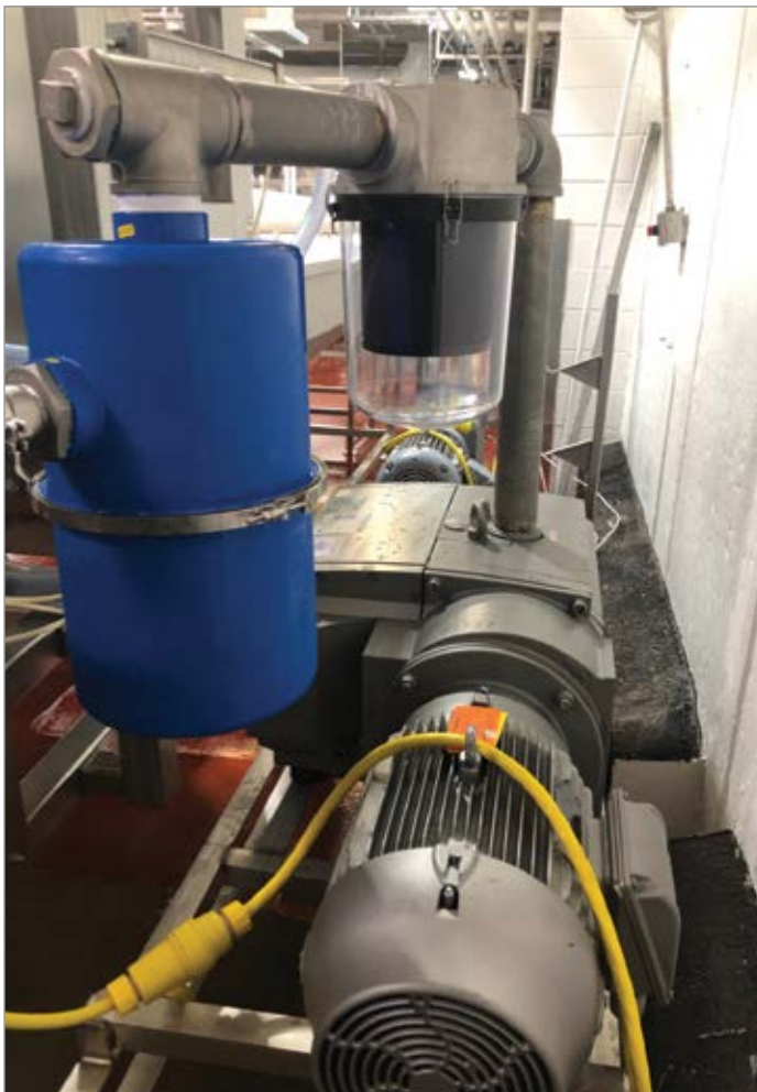
An engineered vacuum solution helps a meat processor save approximately 225 gallons of water per minute during a meat-mixing process – and save on wastewater treatment costs.
