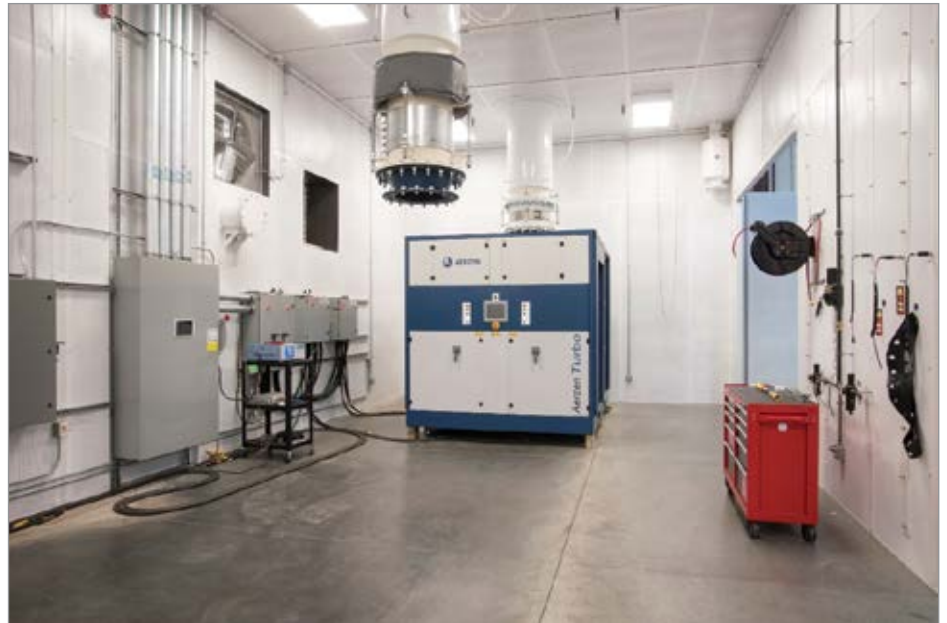
PTC 13 provides procedures for determining the required total operating electrical power of a packaged blower system, termed the “wire-to-air” performance.
