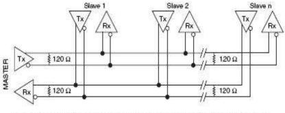
4-Wire Full-Duplex Multidrop Network Using Terminating Resistors
