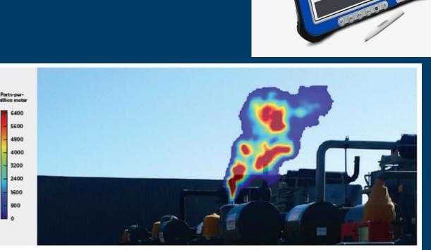
Rebeilion Photonics' Gas Cloud imaging technology provides gas detection videos and images of methane and other gases. The color scale corresponds to gas concentration
