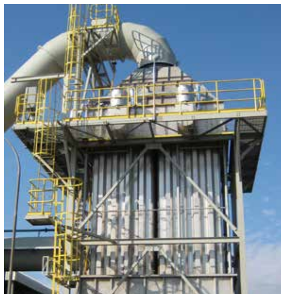
Wet ESP on mineral wool production
