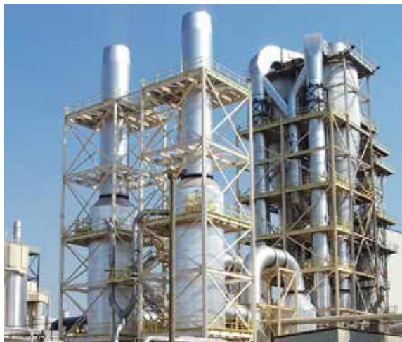
Packed towers for gas absorption
