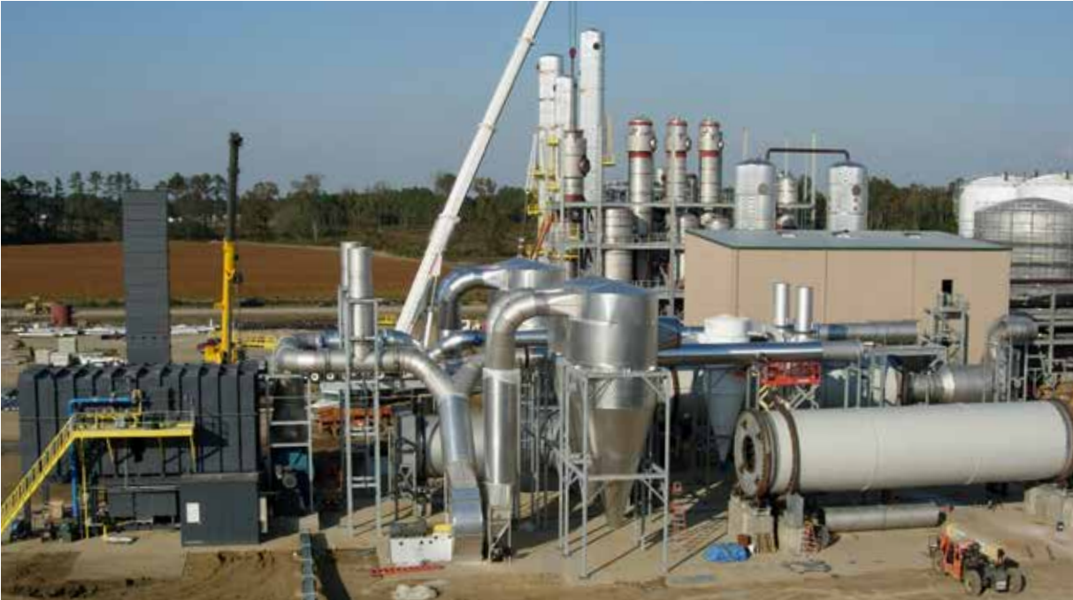
Turnkey supply: RTO, rotary drum dryers, cooler, cyclones and interconnecting ductwork and supports
