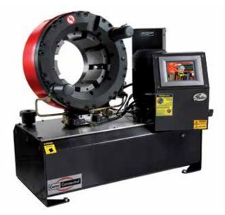
The GC96<sup>™</sup> crimper is capable of crimping up to 6 inch ID industrial hose. The Large crimper head allows industrial hose assemblies to be made with a variety of terminations using crimpable ferrules and sleeves. The GC96<sup>™</sup> crimper has additional versatility since in conjunction with optional spacer dies and GC32–XD<sup>™</sup> dies; it can make Gates hydraulic hose assemblies also.
