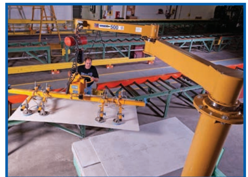
A 500-pound Spanco Freestanding Articulating Jib Crane with a vacuum attachment for easy lifting.
