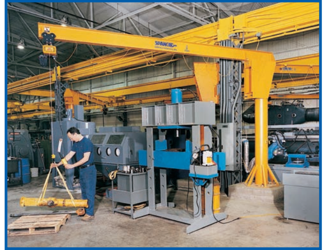
A 1-ton Spanco Freestanding Jib Crane used for shipping and assembly.
