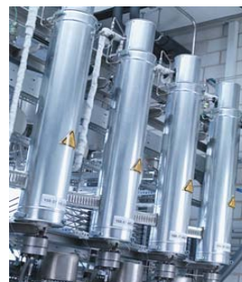
Parallel bench scale test units
