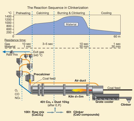
The presence of both exothermic and endothermic chemical reactions makes the cement kiln process unstable. This means that achieving an ideal temperature profile through the kiln is
